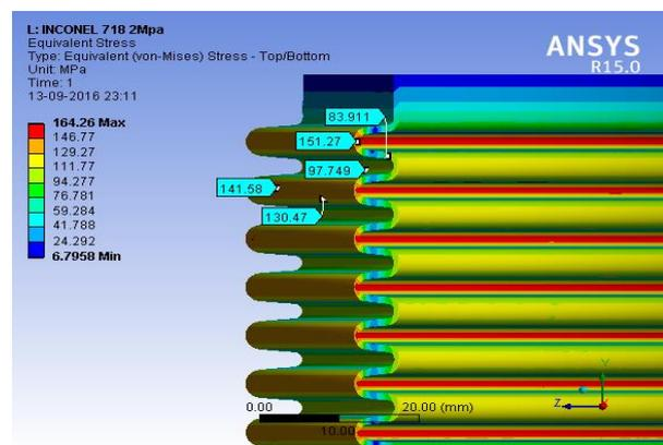
Fig. 19 Stress distribution at Pressure 20 Bar
