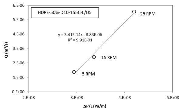
**Fig. 7** Volumetric flow rate vs.  $\Delta P/L$  for the composite containing HDPE5620 as the polymer matrix and 50wt% of wood content (Die temperature: 155°C, die length to diameter ratio: 5, die diameter: 10mm)
