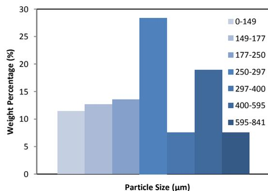
**Fig. 1** Particle size distribution of wood
