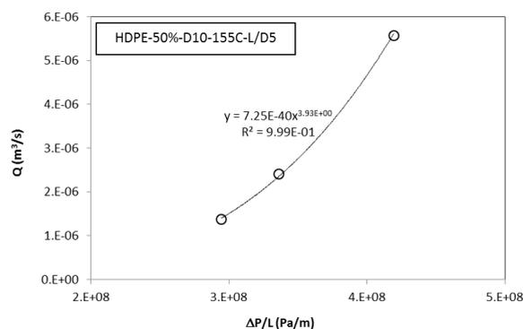
**Fig. 6** Volumetric flow rate vs.  $\Delta P/L$  for the composite containing HDPE5620 as the polymer matrix and 50wt% of wood content (Die temperature: 155°C, die length to diameter ratio: 5, die diameter: 10mm)
