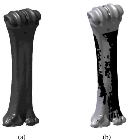
Fig. 12 (a) Point clouds of COMET5™ scanner, (b) consistency of point clouds with output of the developed program as a color coded image
