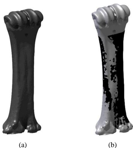
**Fig. 12** (a) Point clouds of COMET5<sup>TM</sup> scanner, (b) consistency of point clouds with output of the developed program as a color coded image
