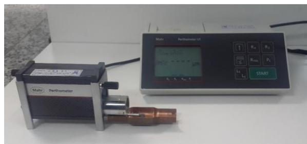
**Fig. 5** Roughness measuring
