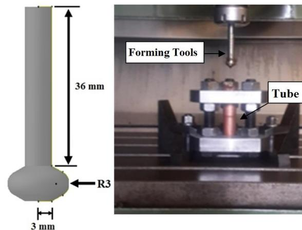
Fig. 3 (a) the forming tool, (b) experimental setup
