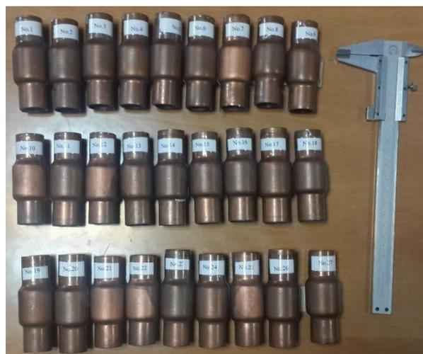
**Fig. 4** Formed specimens using the rotary tool
