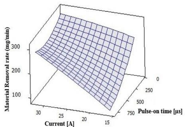
**Fig. 5** Response surface of MRR in terms of current and pulse-on time
