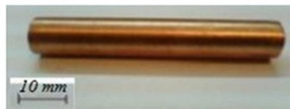
**Fig. 1** EDM milling tool
