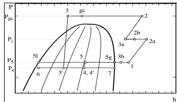
Fig. 4 P-h diagram of new multi-inter-cooling two-stage TRCC cycle with ejector and internal heat exchanger
