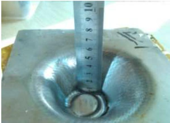
**Fig. 11** Maximum fracture height with tool diameter of 10 mm, step size of 0.25 mm and feed rate of 1800 mm/min in BS mode
