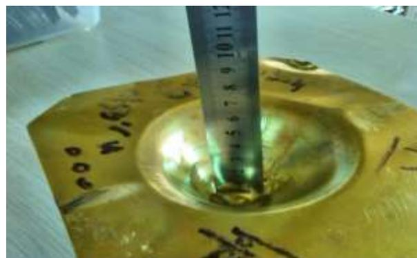
**Fig. 9** Maximum fracture height with tool diameter of 10 mm, step size of 0.5 mm and feed rate of 1000 mm/min in BS mode
