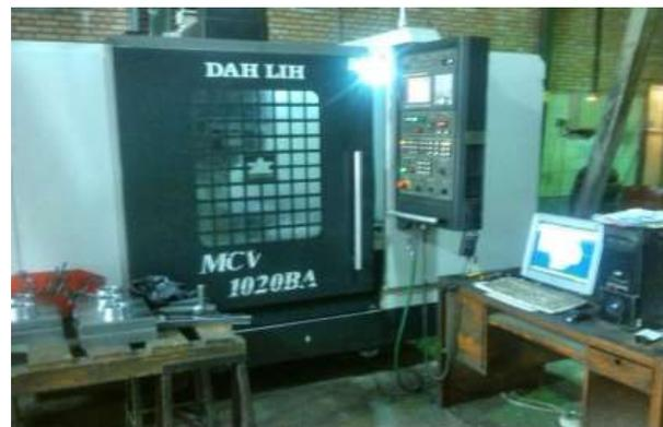
Fig. 1 Image of CNC machine used in incremental forming process tests
