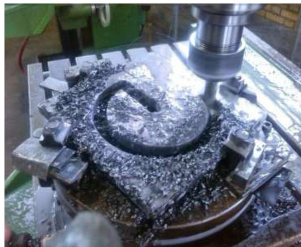
Fig. 2 Construction of the top plate and fixture clamp or mold
