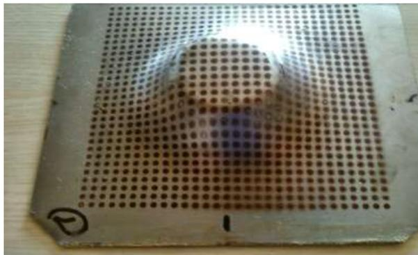
**Fig. 8** An example of carved and formed circles on the sheet after incremental forming
