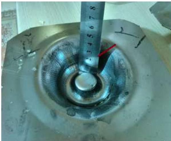
**Fig. 12** Minimum fracture height with tool diameter of 20 mm, step size of 0.75 mm and feed rate of 1800 mm/min in SB mode
