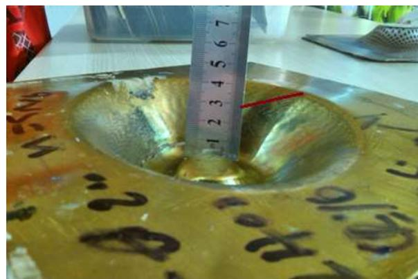
**Fig. 10** Minimum fracture height with tool diameter of 20 mm, step size of 0.5 mm and feed rate of 2400 mm/min in BS mode. Looking at these tables, parameters associated with the maximum and minimum of fracture angles and fracture height during SB and BS modes could be found.
