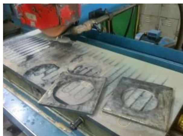
Fig. 3 The grinding clamp plates and the bottom plate during the process of making fixture – mold
