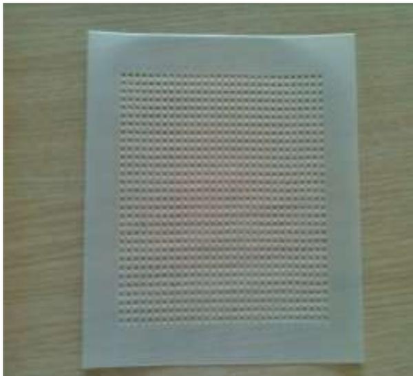
Fig. 5 The stencil designed to make circles with a diameter of 3 mm on the sheet
