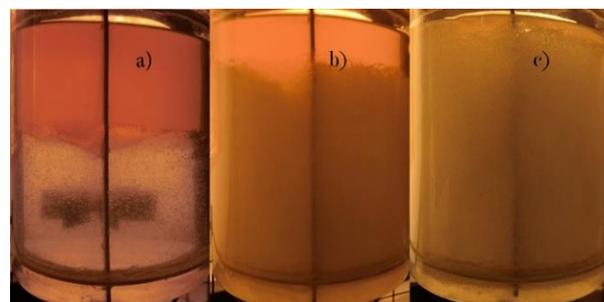
**Fig. 3** Mixing region for off-bottom clearance of 7 cm and baffle width of 21 mm a) impeller speed of 100 rpm, b) impeller speed of 150 rpm, c) impeller speed of 200 rpm.
