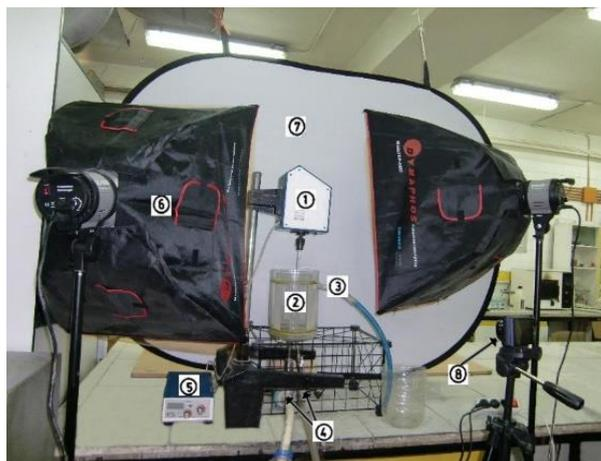
**Fig. 2** Mixer laboratory scale setup (1: mixer, 2: mixer vessel 3: outlet, 4: organic and aqueous inlets, 5: mixer controller 6: flash projector, 7: reflecting surface)
