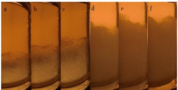
**Fig. 9** Mixing region and flow hydrodynamics in impeller speed of 150 rpm, a) clearance of 5 cm b) clearance of 6 cm c) clearance of 7 cm d) clearance of 8 cm e) clearance of 9 cm e) clearance of 10 cm
