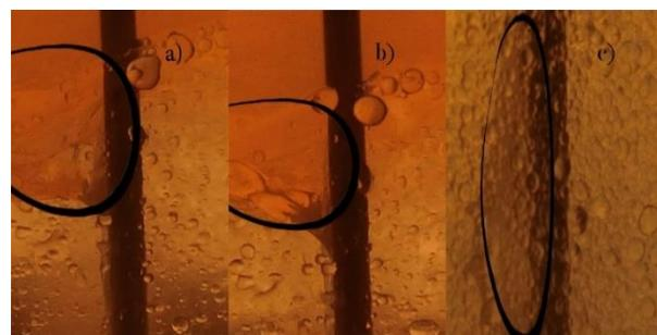
**Fig. 4** Dead zone after baffle a) impeller speed of 100 rpm, b) impeller speed of 150 rpm, c) impeller speed of 200 rpm.
