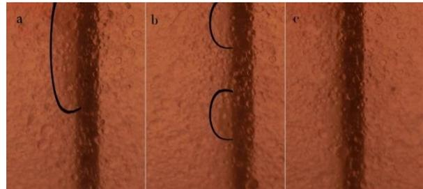
**Fig. 8** Dead zone after baffles in impeller speed of 200 rpm a) impeller diameter of 6 cm, b) impeller diameter of 7 cm, c) impeller diameter of 8 cm.
