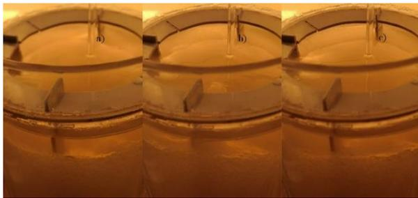
**Fig. 6** Turbulence around baffle for 3 different impellers a) PTU, b) RT, c) PTD
