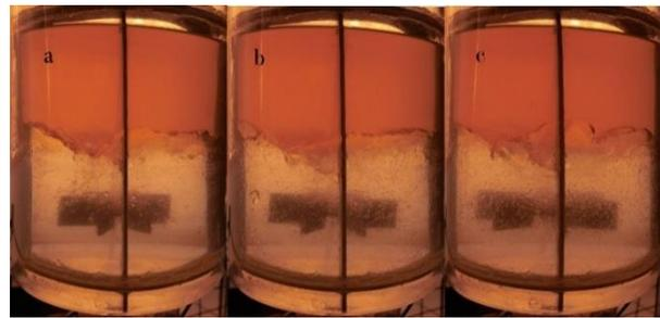
**Fig. 7** Mixing region in impeller speed of 100 rpm a) impeller diameter of 6 cm, b) impeller diameter of 7 cm, c) impeller diameter of 8 cm.
