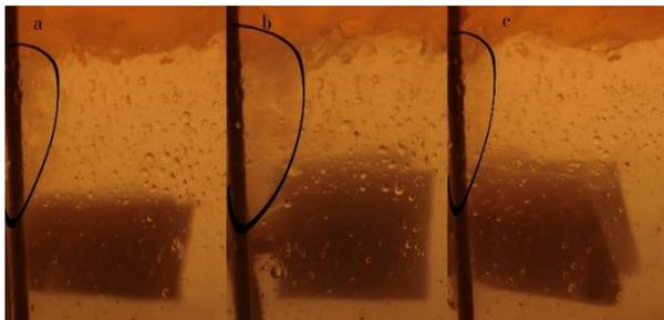
**Fig. 5** Suction region in 3 different impeller type; a) PTU, b) RT, c) PTD
