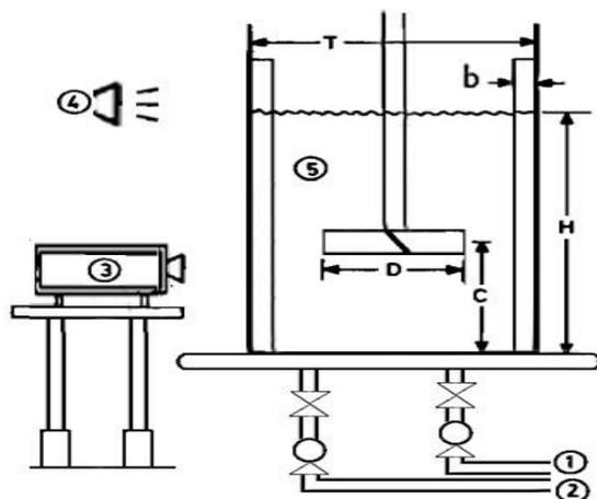
**Fig. 1** Mixer setup schematic and geometry relations ( $H=1.2T=10b=3D=3C$ ) (1,2: organic and aqueous inlets, 3: camera, 4: lighting system, 5: mixer vessel) (H: effective tank height, T: tank diameter, b: baffle width, D: impeller diameter, C: impeller off-bottom clearance)
