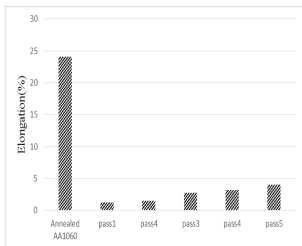
**Fig. 5** Variations of the elongation value of AA1060/Al<sub>2</sub>O<sub>3</sub> composites with the Warm-ARB passes
