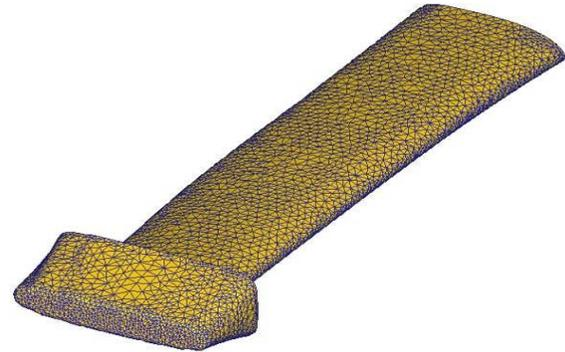
**Fig. 5** Meshed view of modified 0.1 v preform**Table 6** Number of mesh elements
