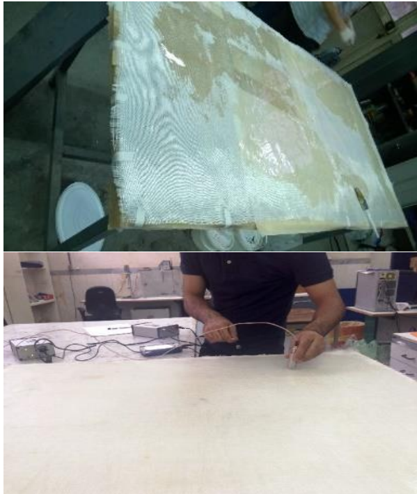
Fig. 4 Producing composite plates and performing Impact-Echo Test
