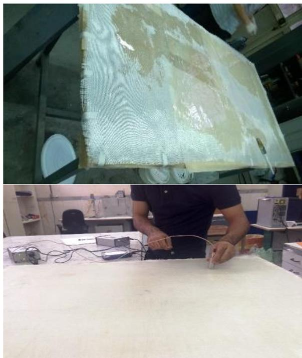
Fig. 4 Producing composite plates and performing Impact-Echo Test
