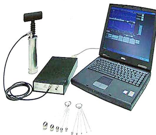
Fig. 2 A simple Impact-Echo system
