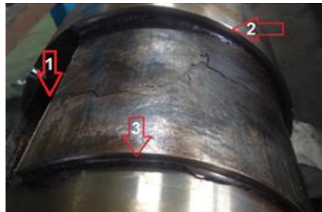
Fig. 28 The fractured gear shaft
