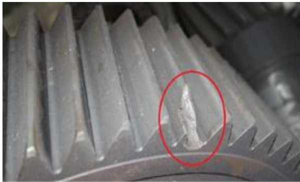
Fig. 3 The lone damaged dent on the gear
