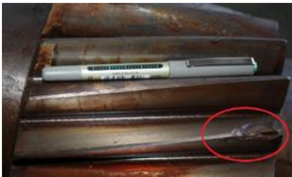
Fig. 4 The damaged dent on the pinion
