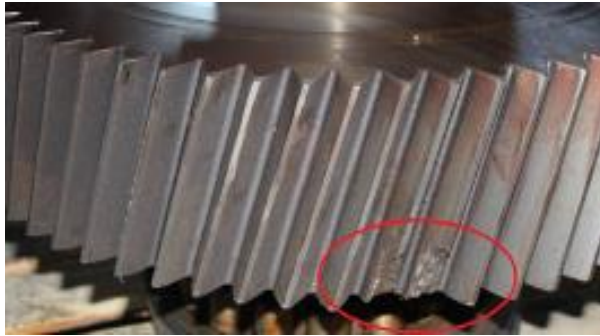
Fig. 2 Two neighbouring damaged dents on the gear
