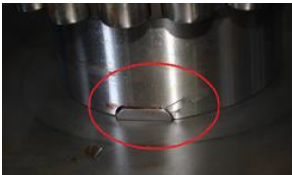
Fig. 5 Damaged location on the shaft
