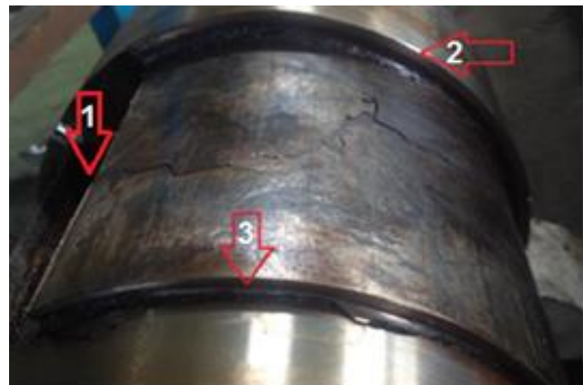
Fig. 28 The fractured gear shaft
