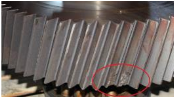
Fig. 2 Two neighbouring damaged dents on the gear
