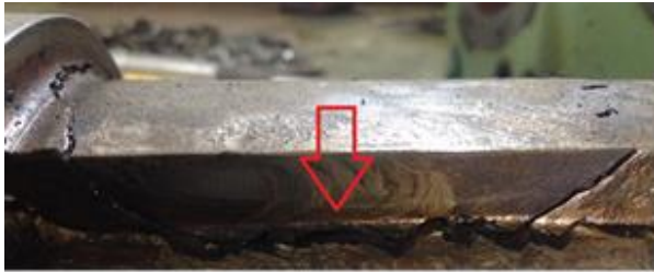
Fig. 39 Crack expansion from stress concentration points in the keyway
