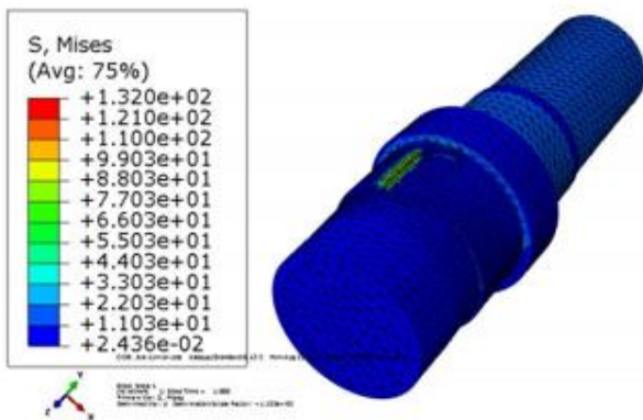
Fig. 30 Stress distribution in redesigned shaft 2
