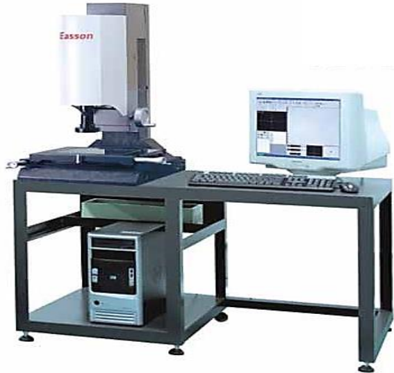
Fig. 4 Image measuring device for wear.
