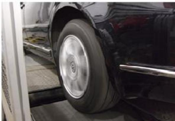
**Fig. 2** The rotary drum for experimental measurement of tire temperature.
