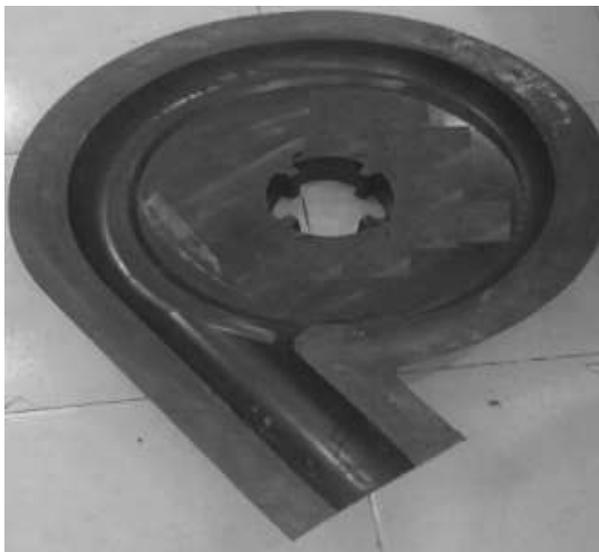
**Fig. 9** Inlet liner made of 1 phr n-ZnO for VASA HD 455-100 pump.
