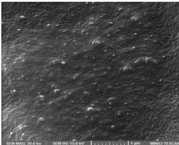
**Fig. 4** FESEM micrograph with magnification X = 30000 of NR/PBR/n-ZnO1.
