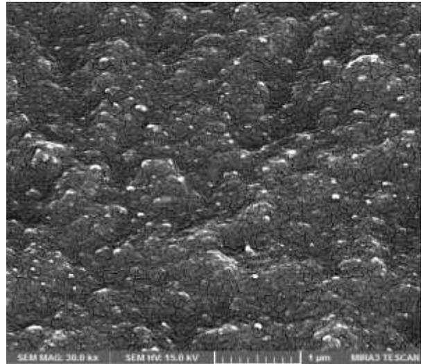
**Fig. 5** FESEM micrograph with magnification X = 30000 of NR/PBR/n-ZnO2.
