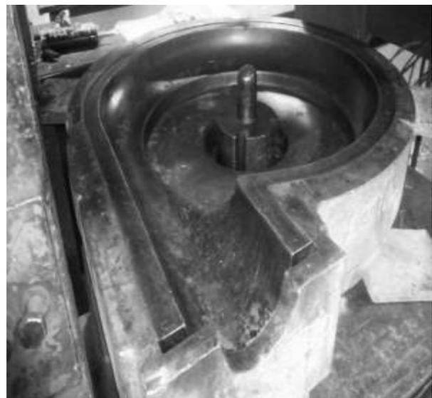
**Fig. 6** Inlet liner mold for VASA HD 455-100 pump.
