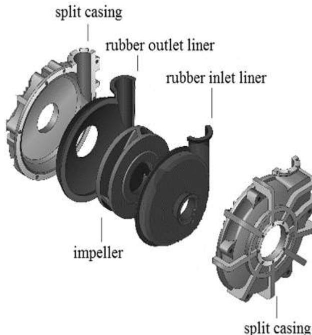
**Fig. 1** Contacting-slurry components of a centrifugal slurry pump including the impeller, inlet and outlet liner.
