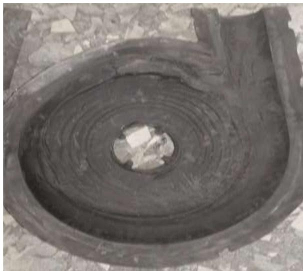
**Fig. 12** Wear of c-liner (liner fabricated with c-ZnO) for VASA HD 455-100 pumps used in hematite plant in Golgohar mining & industrial company.
