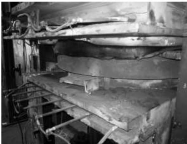
**Fig. 8** The mold was closed with a top plug member and compressed in order to have the material contact at all areas of the mold, while heat and pressure were maintained.
