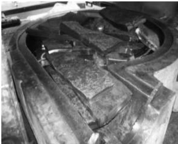
**Fig. 7** The blend was placed in an open mould cavity for VASA HD 455-100 pump.
