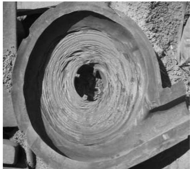
**Fig. 2** Wear of rubber inlet liner for VASA HD 455-100 pumps used in Golgohar mining & industrial company.
