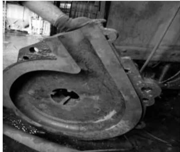
**Fig. 10** Inlet liner was assembled in casing unit of PU302# pump for hematite plant of Golgohar mining & industrial company.
