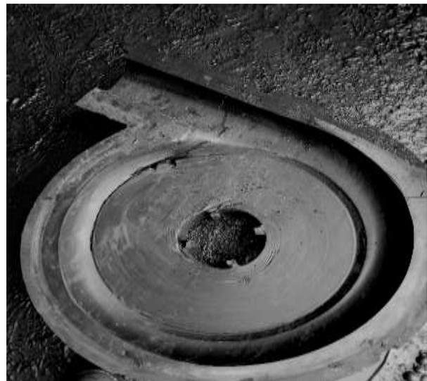
**Fig. 11** Wear of n-liner (liner fabricated with n-ZnO) for VASA HD 455-100 pumps used in hematite plant in Golgohar mining & industrial company.
