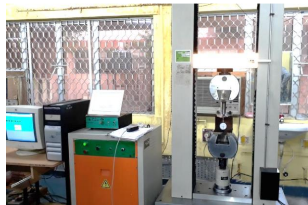
Fig. 5 Experimental Setup of cantilever load test of propeller blade
