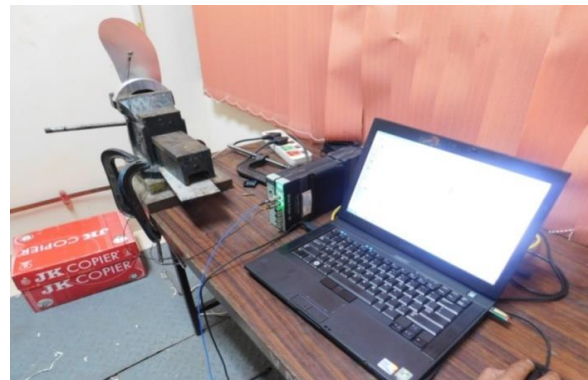
Fig. 13 Experimental setup for impact hammer test method
