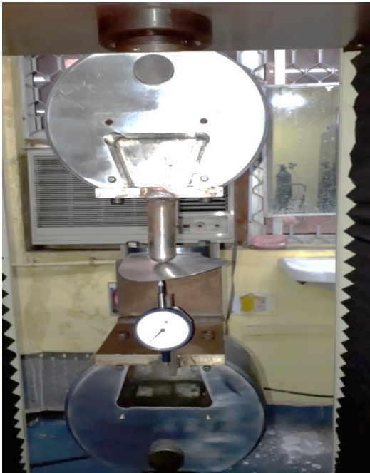
Fig. 6 Assembly of propeller blade and dial gauge to the fixture
