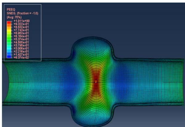
Fig. 9 Finite elements results with optimized loading path.
