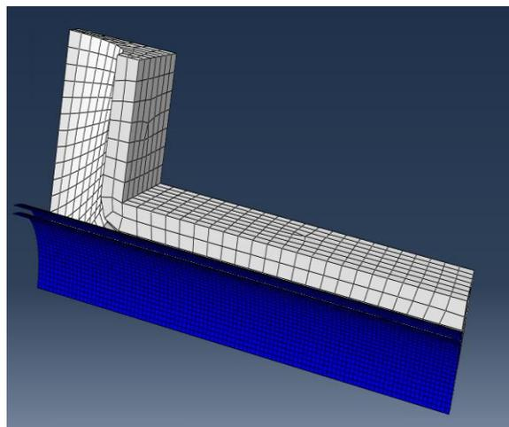
**Fig. 1** Finite element modeling of double-layered X-shape tube hydroforming.
