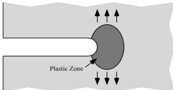
Fig. 5 Plastic zone as a result of overload.
