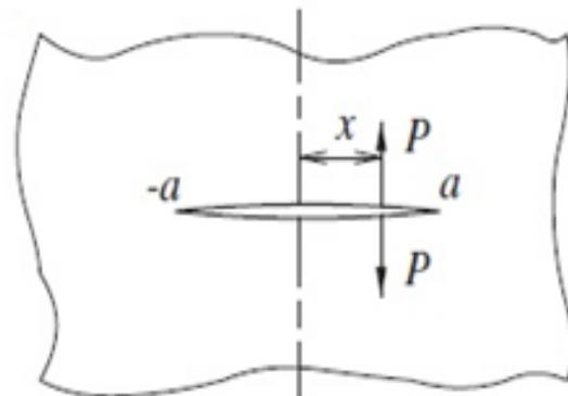
Fig. 4 Configurations of infinite sheet with center.
