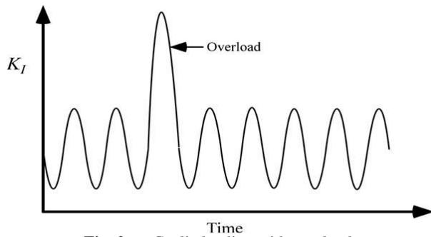
Fig. 2 Cyclic loading with overload.
