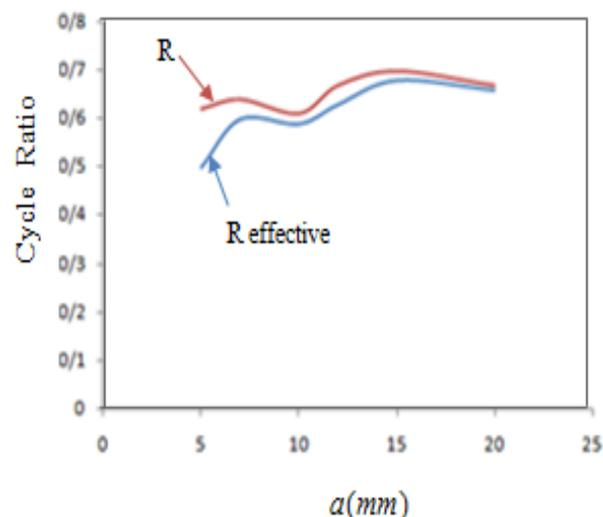
**Fig. 10** Calculated effective stress ratio.
