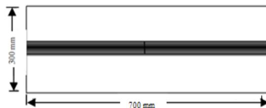
**Fig. 1** Workpiece: dimension and weld position (thickness = 3mm).
