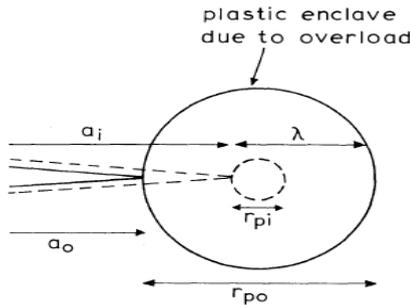
Fig. 7 The model of Wheeler (Situation after overload) [17].
