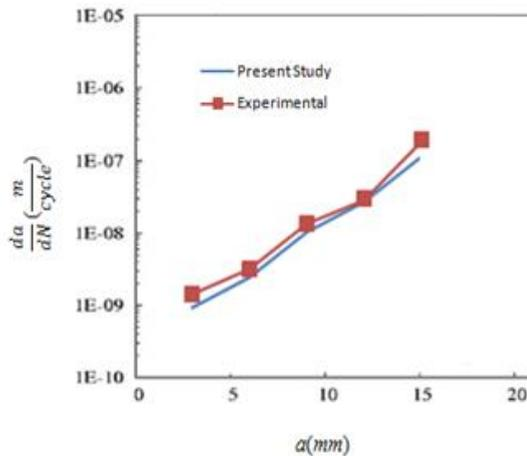
Fig. 11 Predicted and experimental, Fatigue Crack Propagation (FCP).
