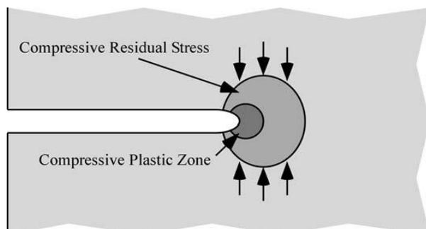
Fig. 6 Residual compressive stresses at crack tip as a result of overload [17].
