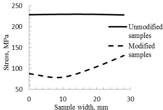
Fig. 18 Von-Mises residual stresses along the weld line.
