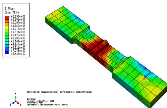
Fig. 13 Von-Mises stress distribution in the sample.
