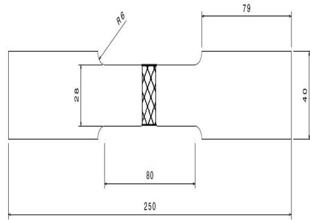
Fig. 2 The view of the fatigue specimen, mm.
