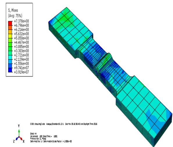
Fig. 15 The distribution of residual stress after TIG-dressing.
