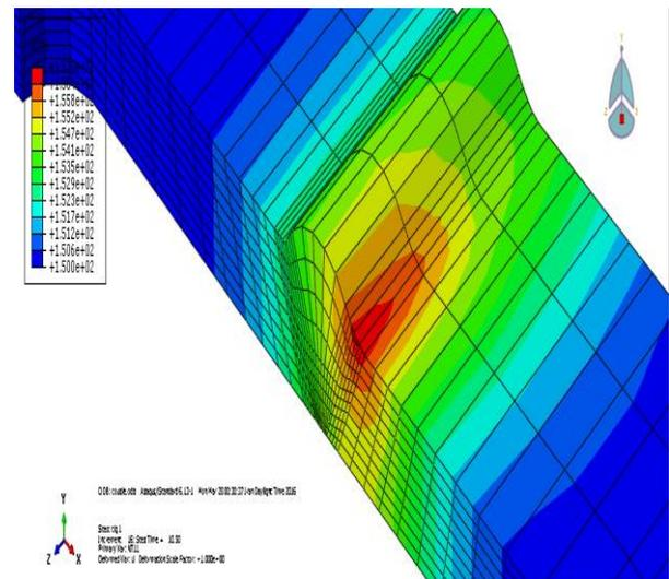
Fig. 14 Applied heat flux to TIG-dressing model.
