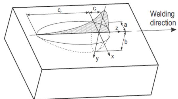
Fig. 7 The elliptical-shaped flux distribution power density [18].
