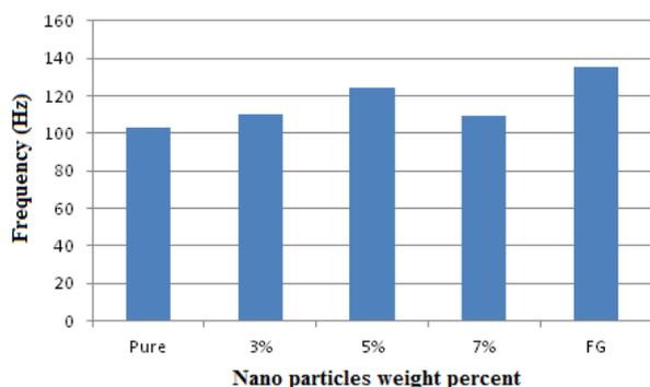
**Fig. 4** The effect of nanoparticles with different weight fractions on the free vibration frequency.
