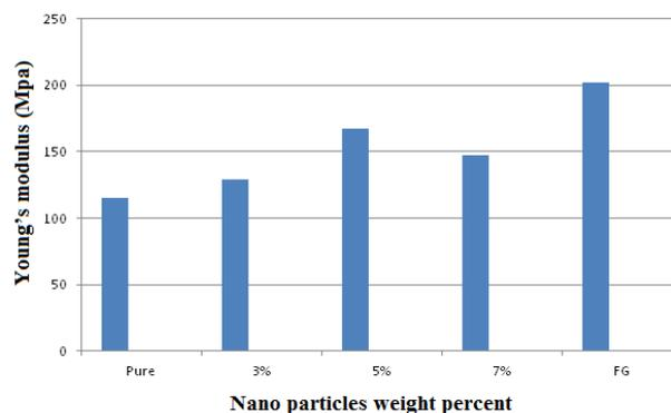
Fig. 1 The Young's modulus of nanocomposites with the different distribution of Nanoparticles.
