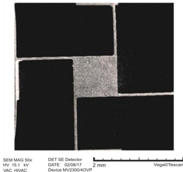
**Fig. 1** A spring-mass structure of a high-g microaccelerometer fabricated using the MicroWEDM process.
