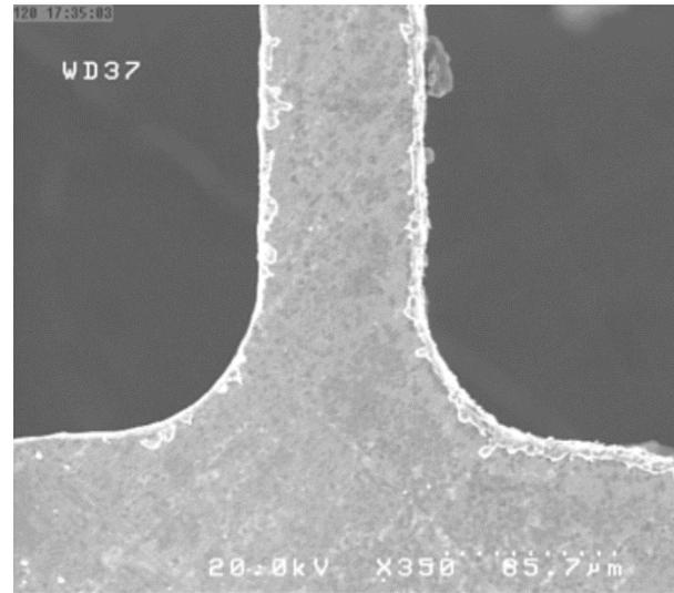
**Fig. 4** SEM image of the micro-feature with optimal dimensional deviation.
