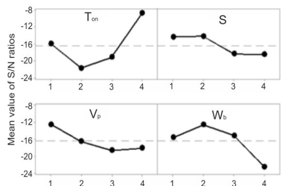
Fig. 3 Effect of different levels of the process parameters on the S/N ratio.
