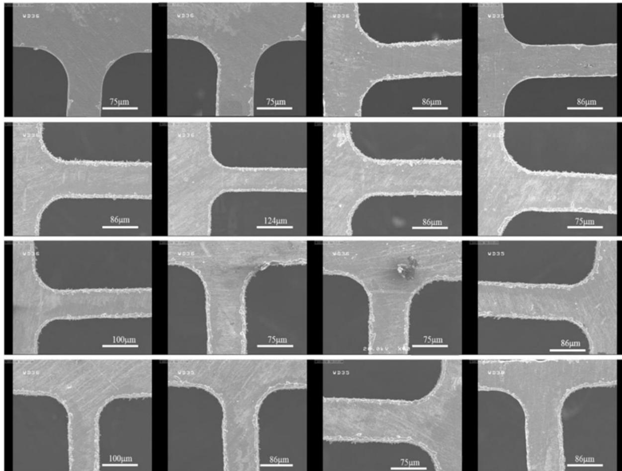
Fig. 2 SEM images of the micro-features based on the experiments layout shown in table 2 (From left to right and top to bottom, corresponding to the number of the experiments).
