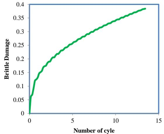
**Fig. 6** Brittle damage variable versus the number of the cycle for 2024 Al alloy under strain 0.04.
