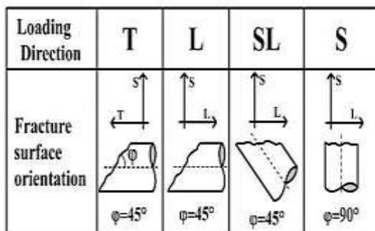
**Fig. 1** 2024 Al alloy fracture cross-section along different direction [16].
