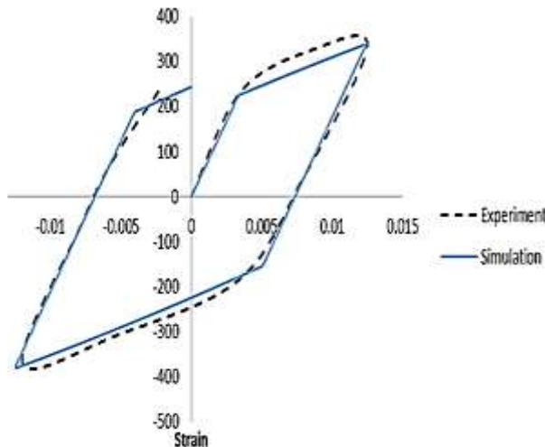
**Fig. 4** Comparison of the stress-strain curve for experimental data [16] & simulation data for 2024 Al alloy under cyclic loading.
