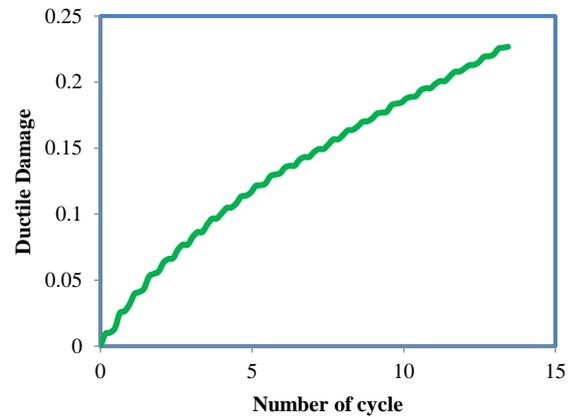
**Fig. 5** Ductile damage variable versus the number of the cycle for 2024 Al alloy under strain 0.04.
