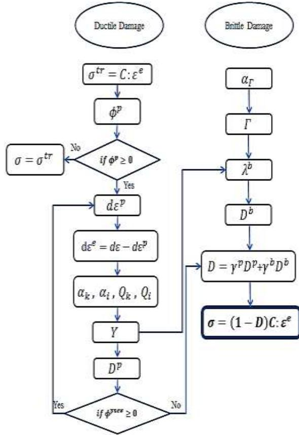
Fig. 2 The Kintzel quasi brittle damage model algorithm.
