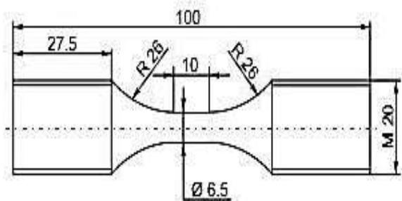
Fig. 3 Geometrical dimension of simulation sample [16].
