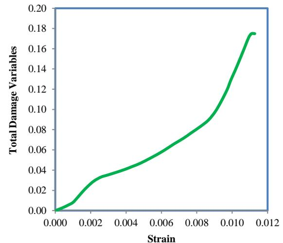
**Fig. 8** Total damage variable versus induce strain for 2024 Al alloy.
