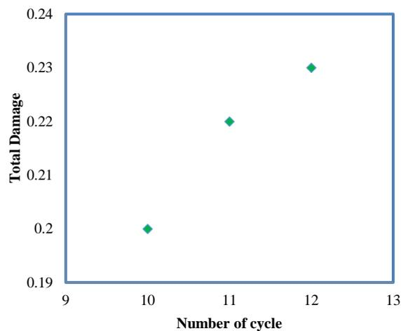
**Fig. 7** Total damage variable versus the number of the cycle for 2024 Al alloy under strain 0.04.
