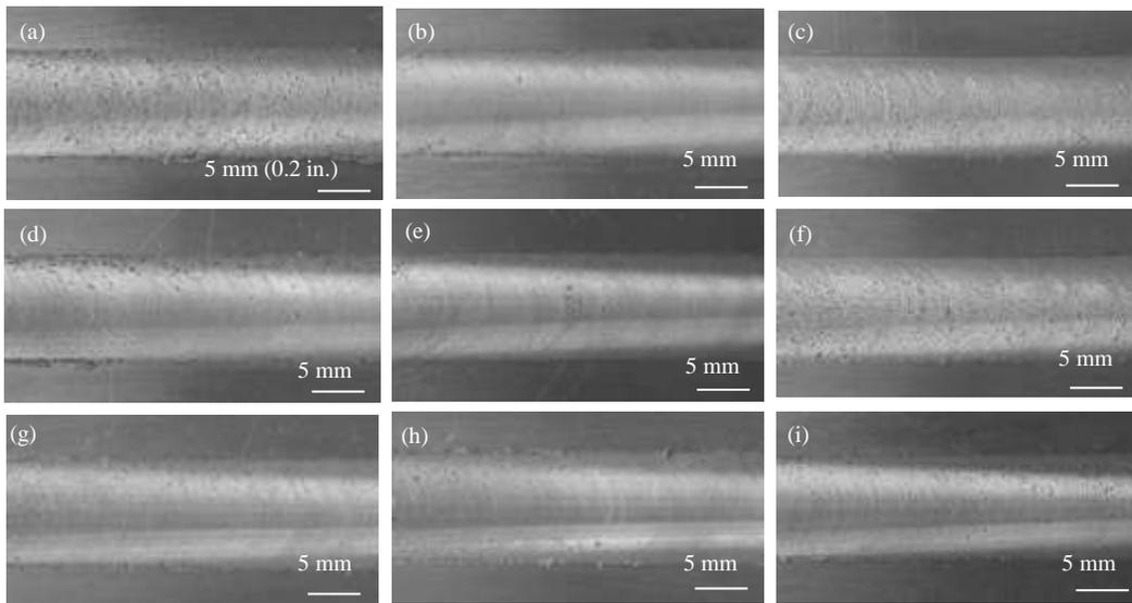
**Fig. 5** Welding quality of dissimilar FSW joints at suitable combinations of tool rotational and welding speeds: (a): 800/63, (b): 800/100, (c): 800/160, (d): 1000/63, (e): 1000/100, (f): 1000/160, (g): 1600/63, (h): 1600/100 and (i): 1600/160.
