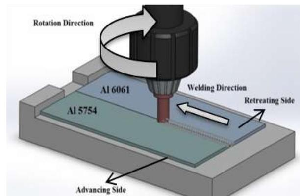
**Fig. 1** Schematic view of conducted dissimilar Friction Stir Welding.
