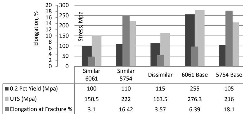
Fig. 11 Mechanical properties of the base alloys, similar and dissimilar joints, at 1000 rpm, 100 mm/min (3.94 in./min).
