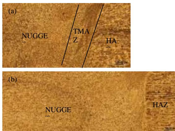
**Fig. 16** Comparison of grain size between nugget and adjacent zones on advancing side: (a): 800 rpm, 63 mm/min (2.48 in./min) and (b): 1600 rpm, 63 mm/min (2.48 in./min), with magnification of 50 times.
