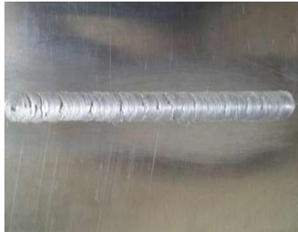
Fig. 4 Defected joint at unsuitable speeds combination.
