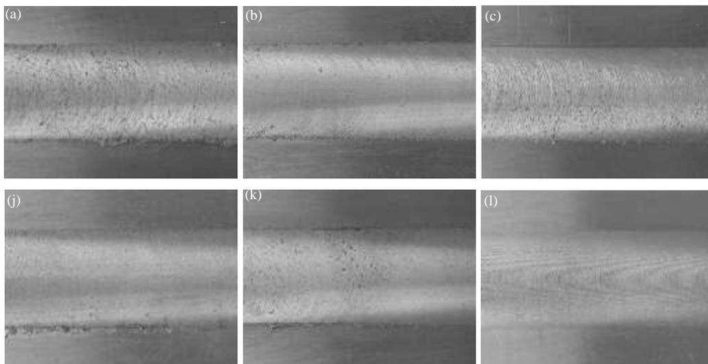
**Fig. 7** Welding quality of dissimilar FSW at suitable combination of rotational and welding speeds – Al 5754 on advancing side: (a): 800/63, (b): 800/100, (c): 800/160, Al 6061 on advancing side, (j): 800/63, (k): 800/100 and (l): 800/160.
