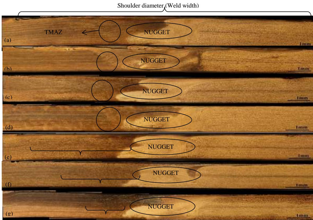
**Fig. 14** Optical macrographs showing the weld zone of the dissimilar FSW joints at various speed combinations etched by modified Poulton's reagent with magnification of 50 times– Al 5754 on the right: (a): 800/63, (b): 800/160, (c): 1000/63, (d): 1000/160, (e): 1600/63, (f): 1600/100 and (g): 1600/160.
