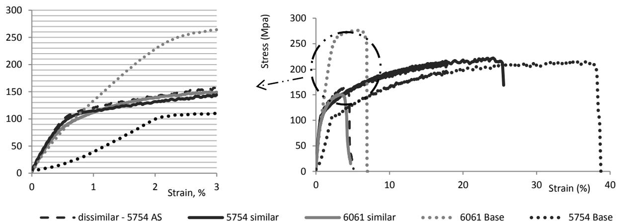
**Fig. 10** The mechanical properties of the similar FSW joints at tool rotational speed of 1000 rpm and welding speed of 100 mm/min (3.94 in./min): (a): tensile strength and (b): 0.2% yield strength point.
