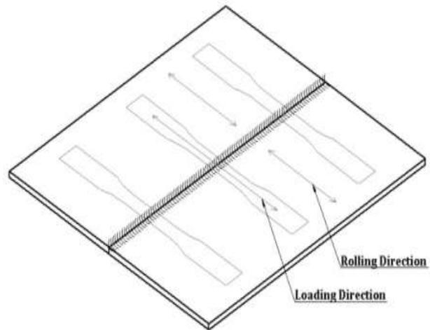
Fig. 3 Prepared tensile specimens according to the ASTM-E8 standard.
