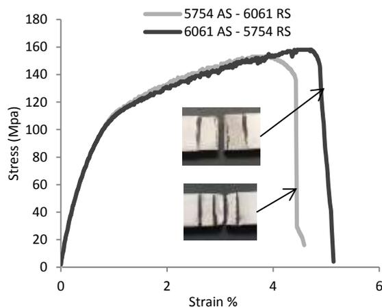
**Fig. 17** Stress-strain curve of dissimilar FSW joints in two situations at 800 rpm, 63 mm/min – advancing side (AS) on the left.
