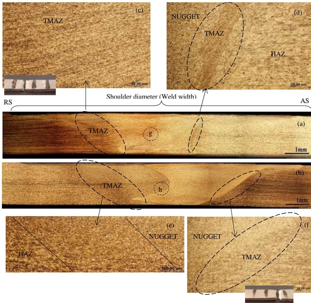
**Fig. 20** Optical macro and micrographs showing weld zones of dissimilar FSW joints at 800 rpm and 100 mm/min, in two different alloy locations: (a): Al 5754 on advancing side (AS), (b): Al 5754 on retreating side (RS), ((a) and (b)): with magnification of 50 times, (c): 100 times, (d): 200 times, (e): 50 times and (f): 200 times.
