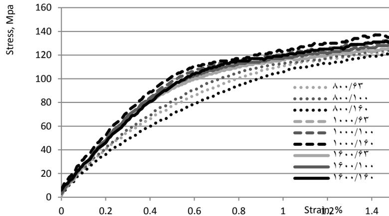
Fig. 12 Comparison of yield strength of dissimilar FSW joints at various speeds combinations.
