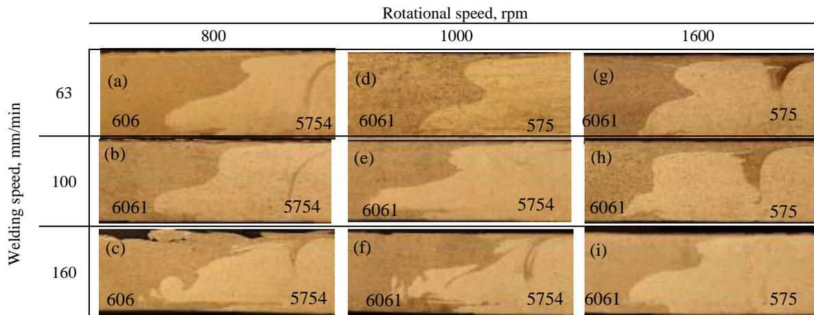
**Fig. 13** Optical macrographs showing the cross section of the dissimilar FSW joints at various speed combinations etched by Modified Poulton's reagent– Advancing side on the right.
