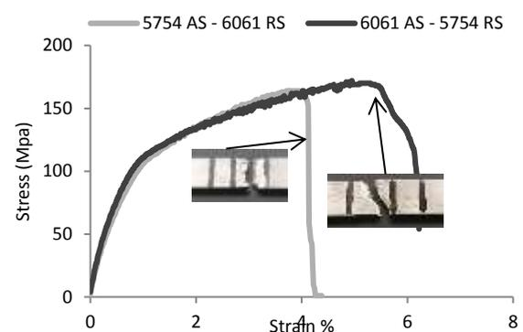
**Fig. 19** Stress-strain curve of dissimilar FSW joints in two situations at 800 rpm, 160 mm/min - advancing side (AS) on the left.
