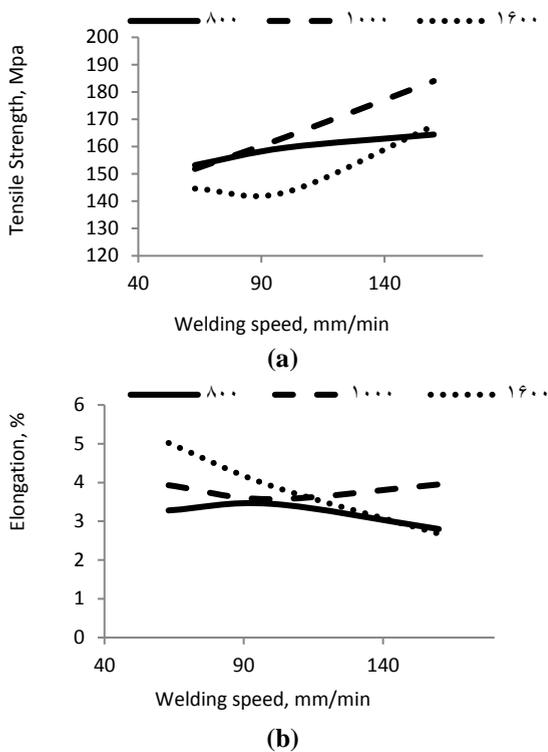
**Fig. 9** (a): Tensile strength and (b): elongation property of joints versus welding speed at three tool rotational speeds of 800, 1000, and 1600 rpm.
