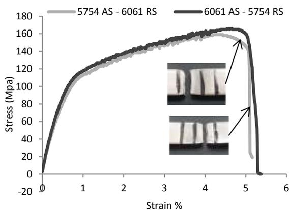
**Fig. 18** Stress-strain curve of dissimilar FSW joints in two situations at 800 rpm, 100 mm/min - advancing side (AS) on the left.
