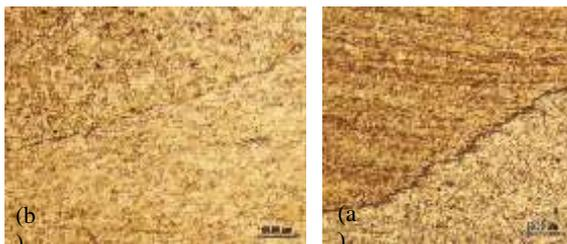
**Fig. 21** The boundary between two alloys in weld nugget: (a): point g and (b): point h, in Fig 20, with a magnification of 100 times.
