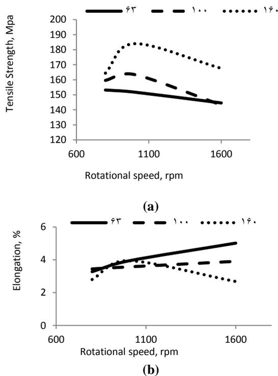
**Fig. 8** (a): Tensile strength and (b): elongation property of joints versus tool rotational speed at three welding speeds of 63, 100 and 160 mm/min (6.3 in./min).
