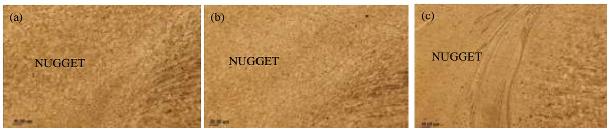
**Fig. 15** Optical micrographs showing TMAZ, HAZ and nugget zone on advancing side of the dissimilar joints welded at 1000 rpm and different welding speeds: (a): 63 mm/min (2.48 in./min), (b): 100 mm/min (3.94 in./min) and (c): 160 mm/min (6.3 in./min), with a magnification of 100 times.
