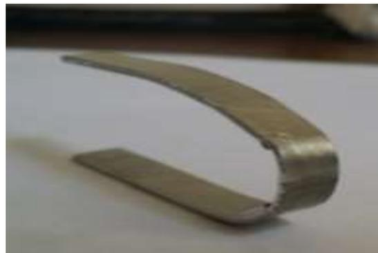
**Fig. 6** The typical root bending test of the dissimilar welds at the welding speed and tool rotational speed of 160 mm/min (6.3 in./min) and 1000 rpm, respectively.
