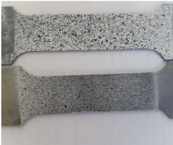
Fig. 5 Two different speckle patterns on the specimens
