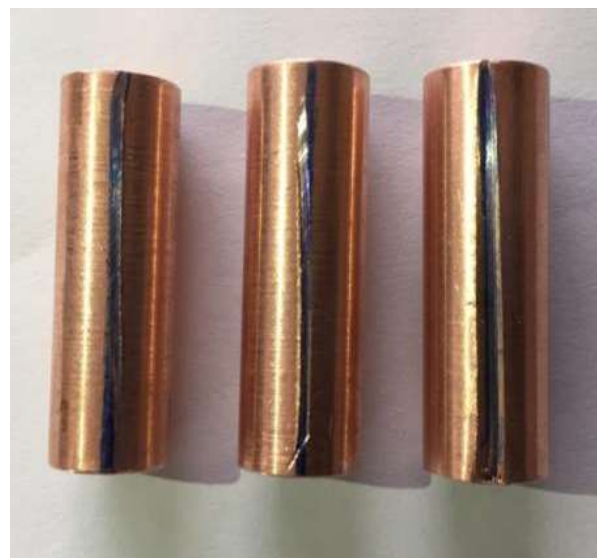
Fig. 4 The lines scribed on SIHPT samples in order to trace a rotation angle.
