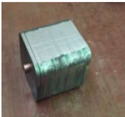
Fig. 2 One of anvils which consists of several steppers (sample is located inside the Steppers).
