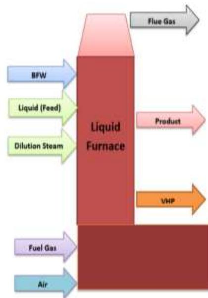
Fig. 3 Streams for a liquid feed furnace.
