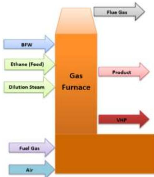
Fig. 2 Streams for a gas feed furnace.
