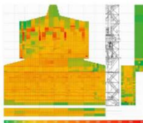
**Fig. 5** Extracted temperature in degrees centigrade for furnace 104 in real condition.
