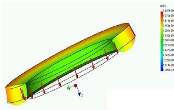
**Fig. 12** Bending of the ring (thickness 10mm) seated on the outer diameter,  $\sigma_{\max}=22.35$  MPa.
