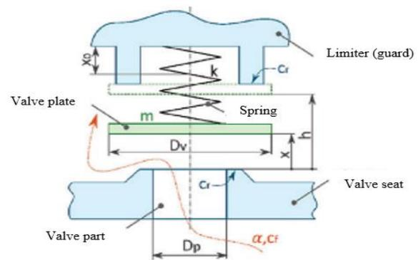
**Fig. 2** Generic Model of a Valve Assembly [7].
