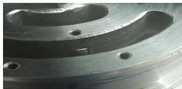
**Fig. 10** Break in the spring compartment from the outside view.
