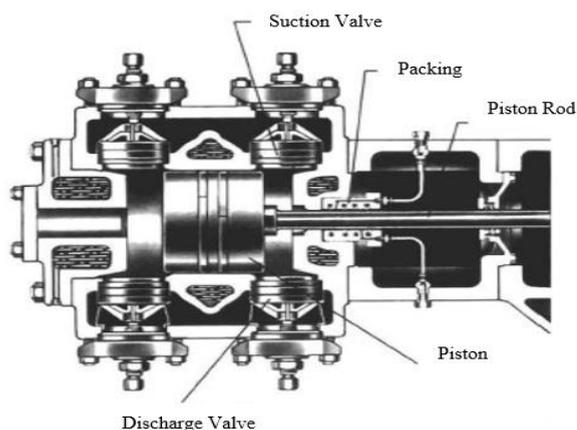
**Fig. 1** The location and method of placing the valve in the compressor [3].
