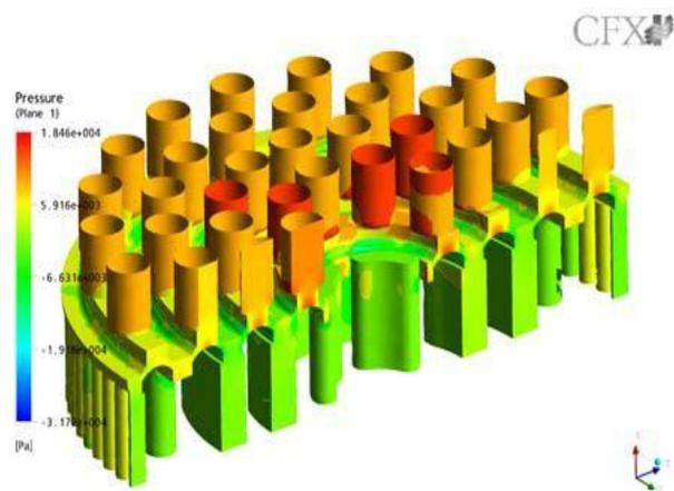
Fig. 16 The fluid pressure in the suction valve (3D view).
