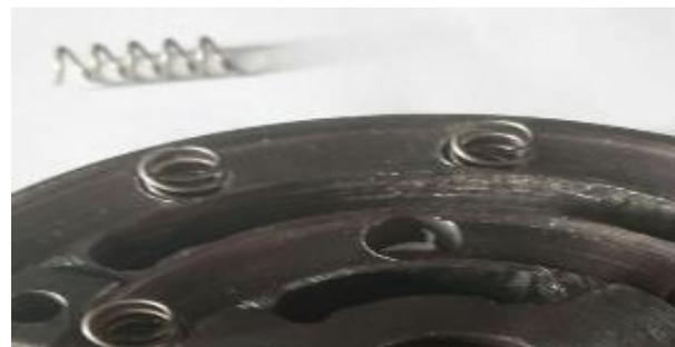
**Fig. 9** Break in the compartment of the spring from the inside view.
