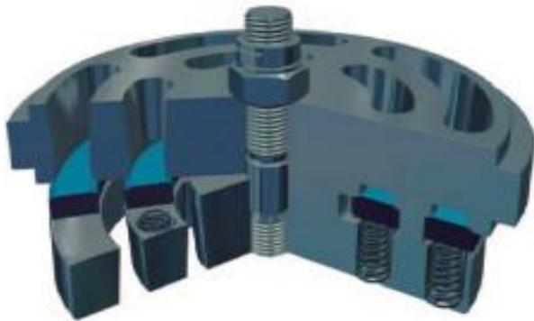
**Fig. 11** Cut-off valve model.
