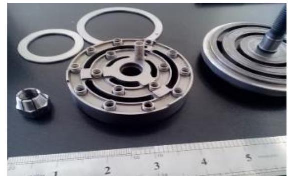
Fig. 7 Elements of ring valve Case Study.
