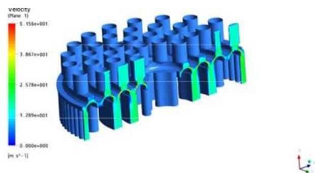
**Fig. 14** The fluid velocity in the suction valve (3D view).
