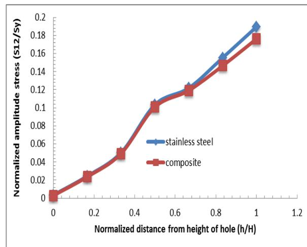
Fig. 17 Dimensional distribution of stress in the direction of the shear in the compartment of the placement of the springs.
