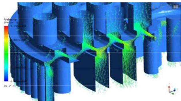
**Fig. 15** The fluid velocity vector in the suction valve (3D view, detail).
