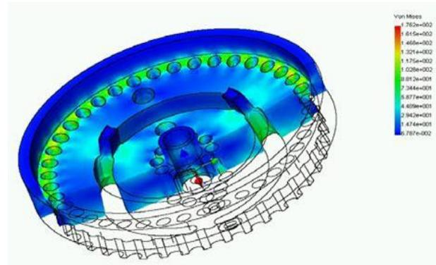
**Fig. 13** Von Mises stresses on the guard,  $\sigma_{\max}=176.2$  MPa.
