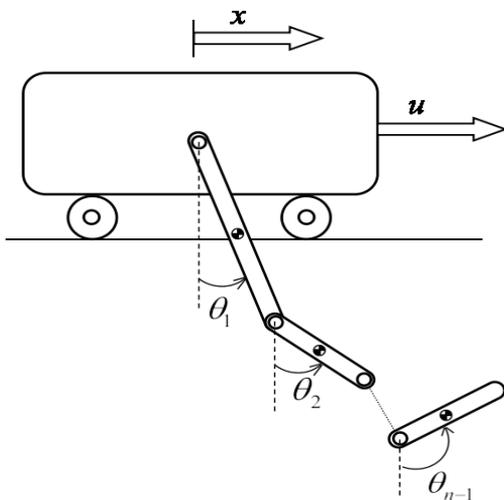
Fig. 1 Schematic view of a classical inverted pendulum with n-1 links.
