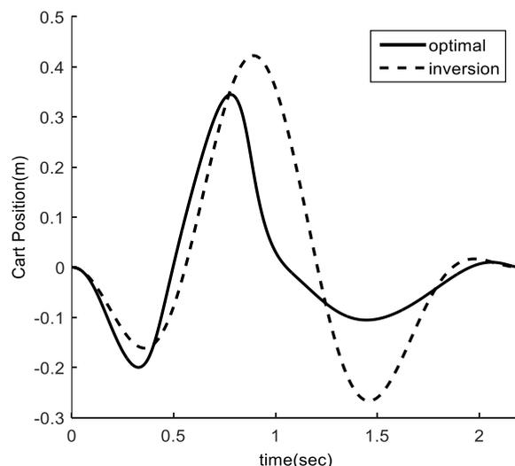
**Fig. 3** Linear position of cart.
