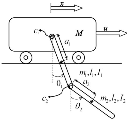
Fig. 2 A double inverted pendulum on a cart.
