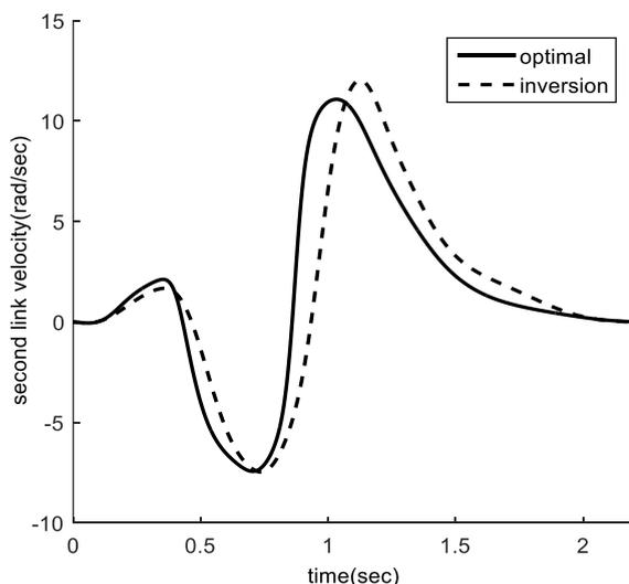
Fig. 8 Angular velocity of the second link.
