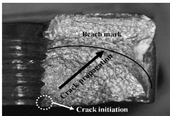
Fig. 7 The fracture surface of the compression hole by means of the optical microscope.
