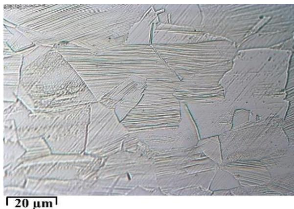
Fig. 1 The austenitic microstructure of LCP.
