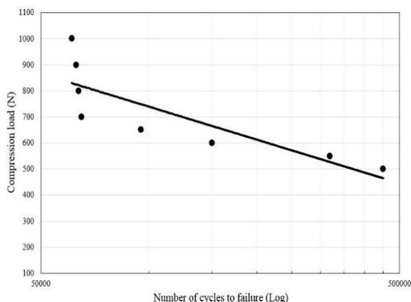
Fig. 5 Relation between compression load and fatigue life cycles.
