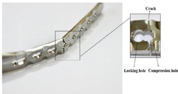
Fig. 6 Location of the fatigue crack at two sides of the compression hole.
