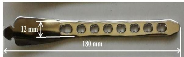
Fig. 2 Test specimen and its dimensions.
