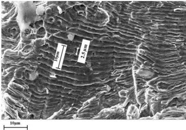
**Fig. 9** Fatigue striation spacing at the middle of the fracture surface.
