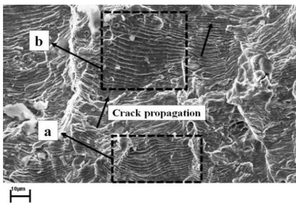
Fig. 8 Fatigue striations near the crack initiation site, (a): shorter striation spacing and (b): longer striation spacing.
