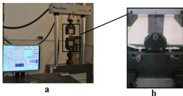
Fig. 4 The fatigue four-point bending test, (a): The Zwick/Roell Amsler HB100 testing machine and (b): The standard four-point bending jig.
