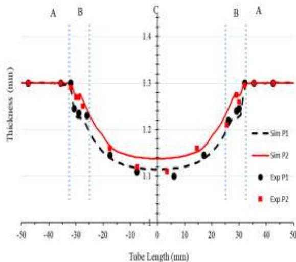
Fig. 9 Thickness distribution in specimens P1 and P2 from experiments and simulation.
