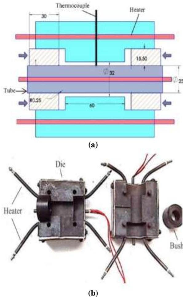
Fig. 1 (a): Schematic of die set designed and (b): the die set made for experimental tests.
