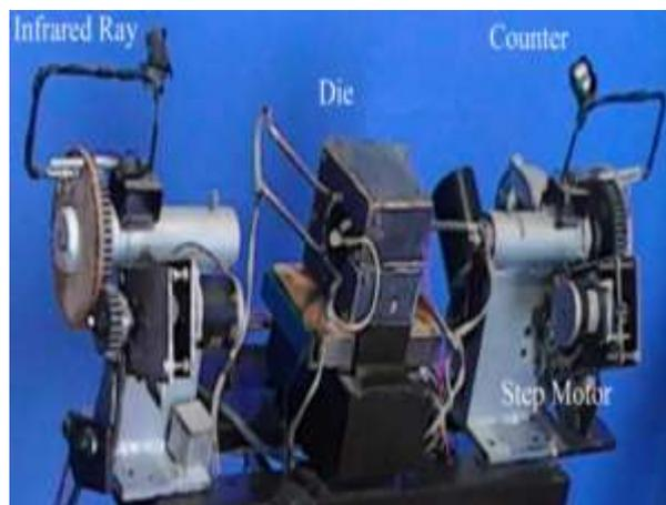
Fig. 2 Equipment set for the hot metal gas forming process with axial feeding.
