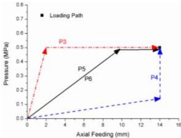
Fig. 4 The loading paths of P3-P6 with an axial feeding condition.
