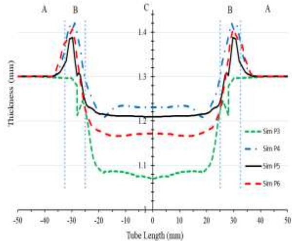
**Fig. 12** Thickness distributions of specimens P3-P4.
