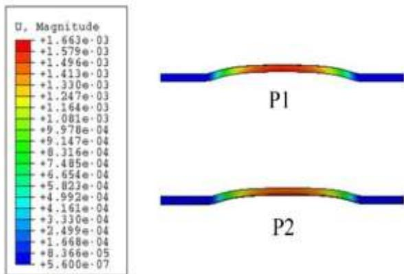
Fig. 8 The radial displacement of specimens P1 and P2 based on simulation results.
