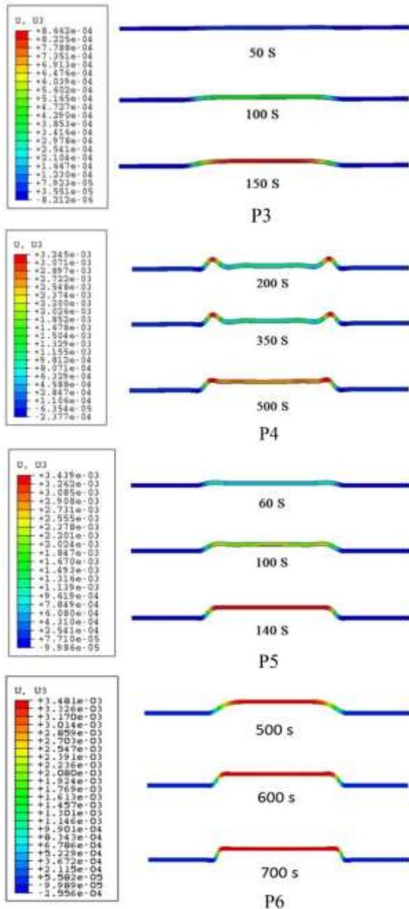
**Fig. 11** The deformation of specimens P3-P6 at different times of forming in terms of radial displacement.
