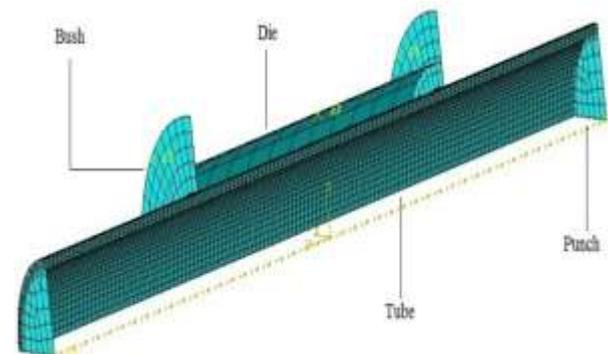
Fig. 3 A quarter model for tube and the die components used in the simulation.
