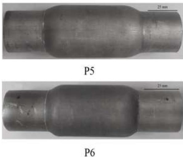
Fig. 13 Specimens P5 and P6 after deformation from experimental tests.
