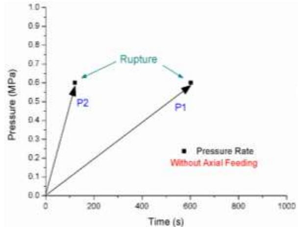
Fig. 6 The pressure rate for the loading paths of P1 and P2.
