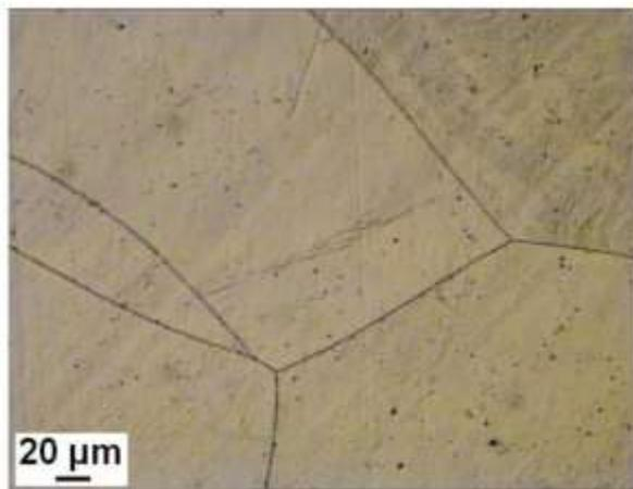
Fig. 2 Microstructure of the as-received pure Mg ingot.
