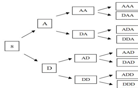
Fig. 1 Three level wavelet packet decomposition [38].
