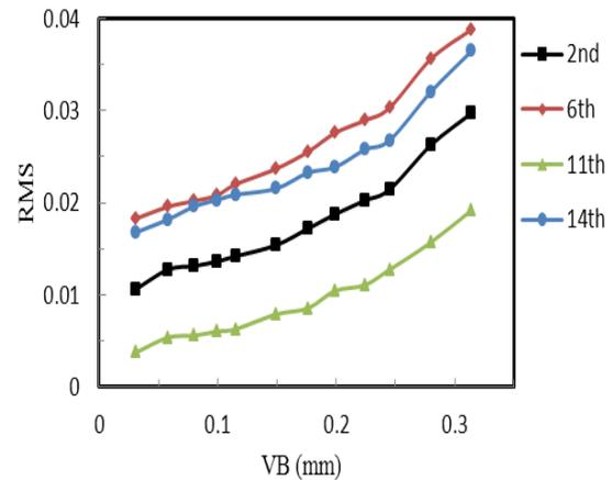
Fig. 7 RMS of wavelet coefficients in selected features for  $v=60$  m/min and  $f=0.02$  mm/rev.
