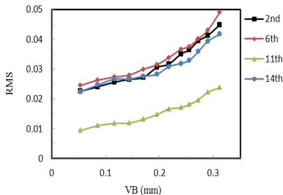
Fig. 10 RMS of wavelet coefficients in selected features for v=80 m/min and f=0.06 mm/rev.
