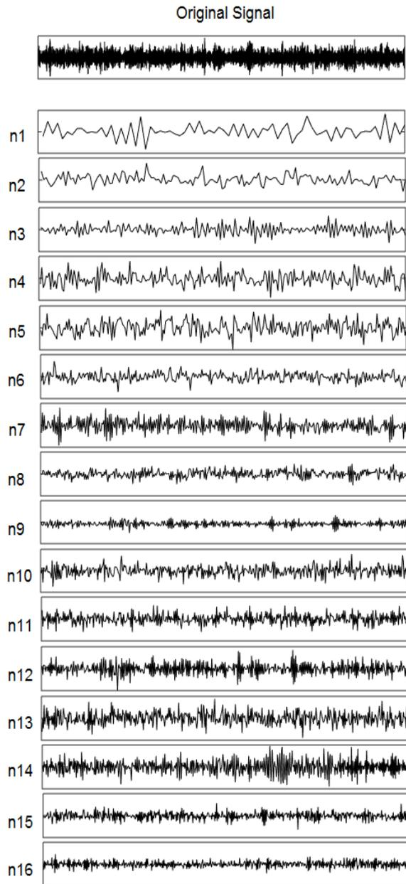
Fig. 6 Captured signal for  $v= 60$  m/min and  $f= 0.04$  mm/rev and decomposed wavelet packets,  $VB=0.27$  mm.
