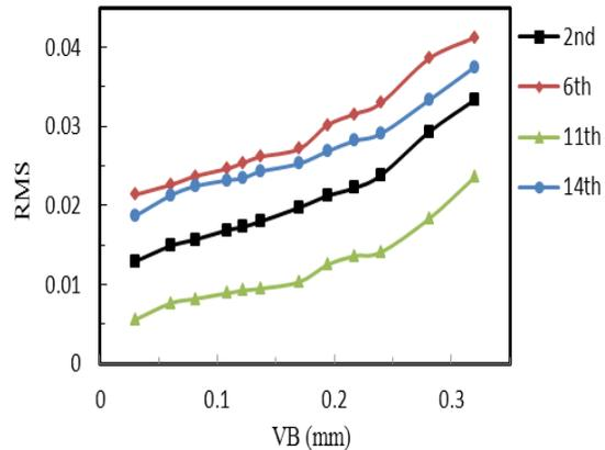
Fig. 8 RMS of wavelet coefficients in selected features for  $v=60$  m/min and  $f=0.04$  mm/rev.
