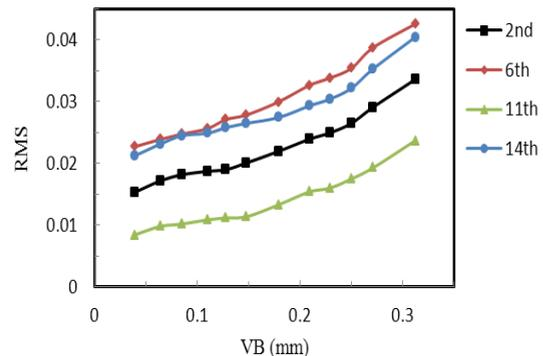
Fig. 9 RMS of wavelet coefficients in selected features for  $v=60$  m/min and  $f=0.06$  mm/rev.
