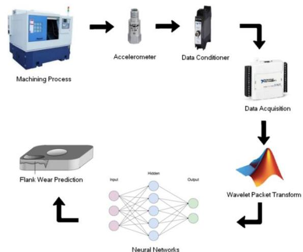
Fig. 2 Schematic diagram of the experimental set-up.
