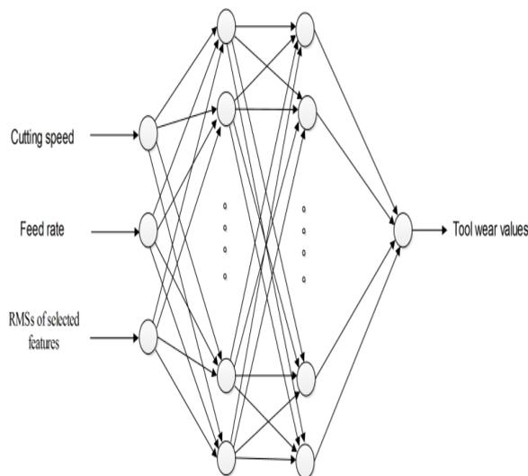
Fig. 4 A schematic view of the trained neural network.
