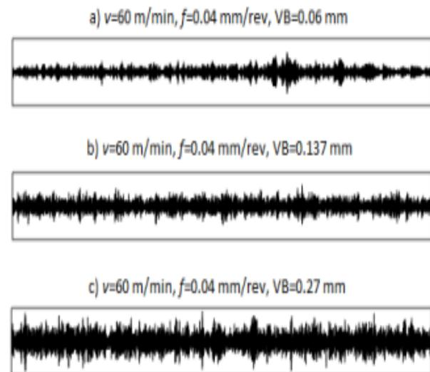
Fig. 5 Captured signals  $v=60$  m/min and  $f=0.04$  mm/rev for different tool flank wear values: (a):  $VB=0.06$  mm, (b):  $VB=0.137$  mm and (c):  $VB=0.27$  mm.
