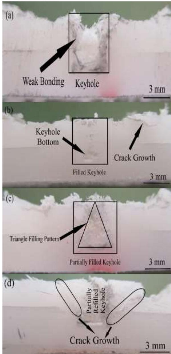
**Fig. 9** Cross-section of TFSSWed specimens: (a): test No. 2, (b): test No. 7, (c): test No. 1, and (d): test No. 4.
