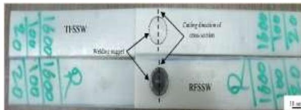
Fig. 6 TFSSWed and RFSSWed specimens.
