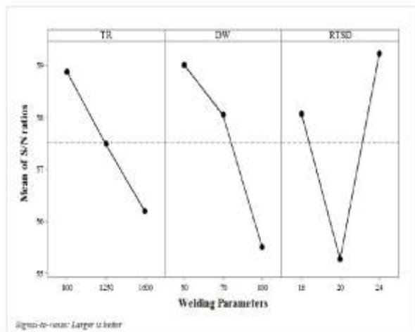
Fig. 5 Main effects plot for S/N ratios of RFSSWed specimens.
