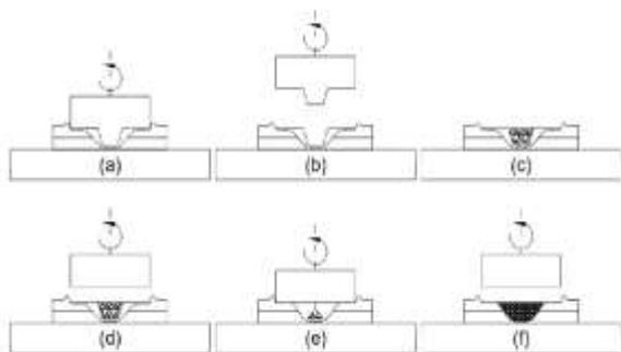
Fig. 1 Schematic illustration of the RFSSW process.
