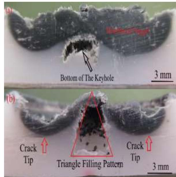
**Fig. 10** The cross-section of the RFSSWed samples: (a): test No. 7 and (b): test No. 1.
