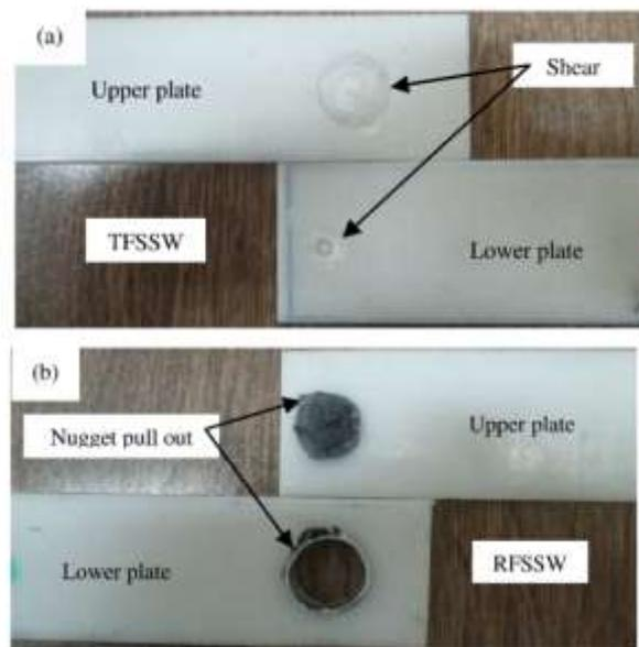
**Fig. 8** Upper and lower sheets after the tensile test: (a): TFSSWed specimen and (b): RFSSWed specimen.
