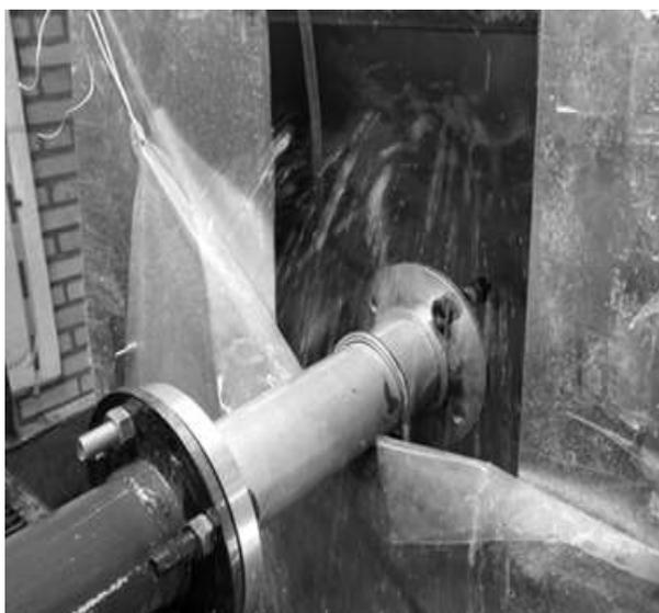
Fig. 10 Constructed turbine while being tested.
