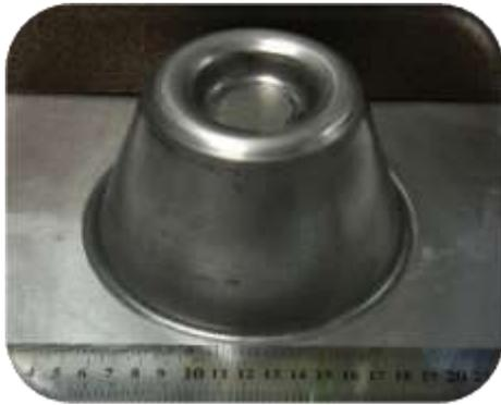
**Fig. 3** The manufactured specimen with two-point incremental forming.
