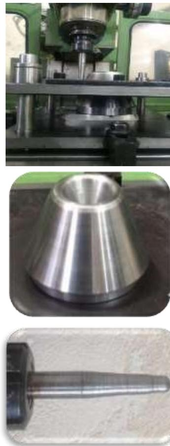
Fig. 2 The die and fixture used in this research drawing.
