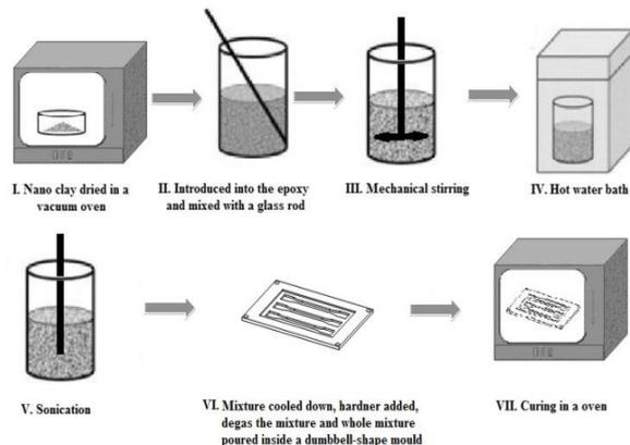
Fig. 1 Preparation procedure for uniform distribution.
