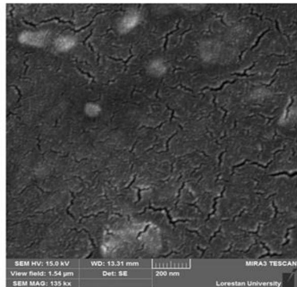
Fig. 3 FESEM image of nanocomposite for uniform distribution.
