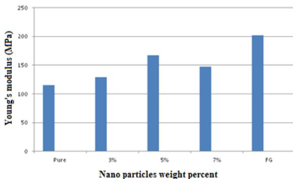
Fig. 6 The Young's modulus of nanocomposites with different distribution of nano particles.
