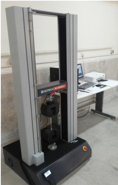
Fig. 5 The Gotech universal testing machine (Model GT-AI5000L).
