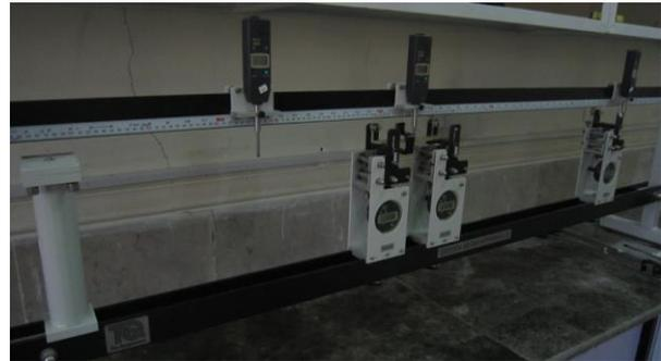
Fig. 9 The beam apparatus TQ (Model SM1004).
