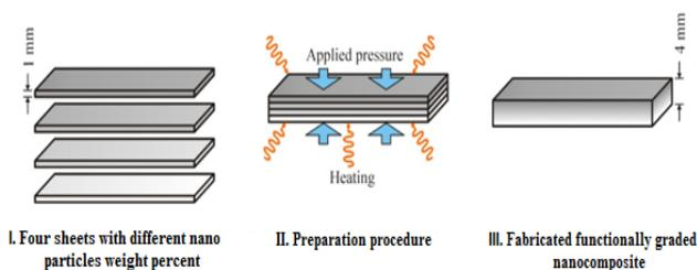
Fig. 2 Preparation procedure for functionally graded distribution.
