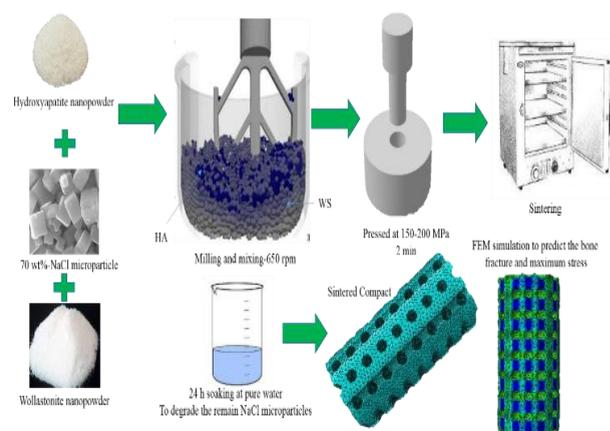
**Fig. 1** Schematic preparation of nHA/CaSiO<sub>3</sub> in this study using space holder technique.
