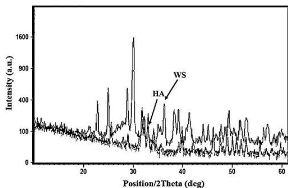
Fig. 2 The XRD comparison pattern of HA, WS, and HA-WS nanocrystalline powder used to fabricate cylindrical scaffold for femur fracture.
