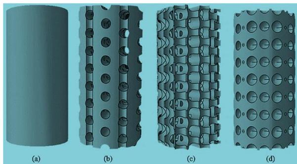
**Fig. 3** (a): Base model without porosity, (b): first porous model, (c): second porous model and (d): spherical porosity model.
