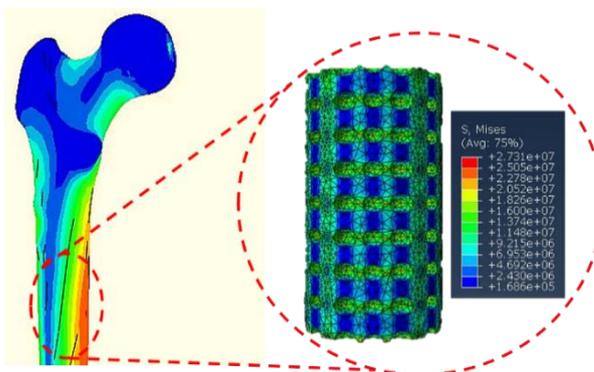
**Fig. 7** Simulation of femur body with Abaqus software with the porous scaffold architecture under various load, the red area shows the maximum stress.
