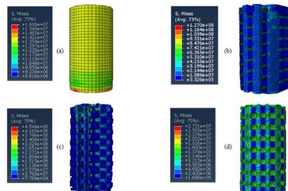
**Fig. 5** Von-mises stress in: (a): base model without porosity, (b): first porous model, (c): second porous model and (d): spherical porosity model.
