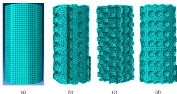
**Fig. 4** Meshed models used for analysis of the porous bio-nanocomposite: (a): cubic mech, (b): non homogenised, (c): randomize and (d): spherical porous architecture.
