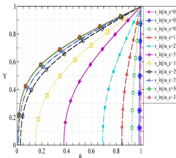
**Fig. 5** Dimensionless temperature profile at the vertical line  $X = 0.5L$  for input Reynolds number  $Re = 1$ ,  $\phi = 0.02$ ,  $B = 0.1$ , and different injection velocities.
