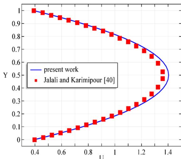
**Fig. 2** Dimensionless velocity profile at the vertical line  $X = 0.6L$  for input Reynolds number  $Re = 10$ ,  $\phi = 0.02$ ,  $B = 0.1$ , and injection Reynolds number of 1.
