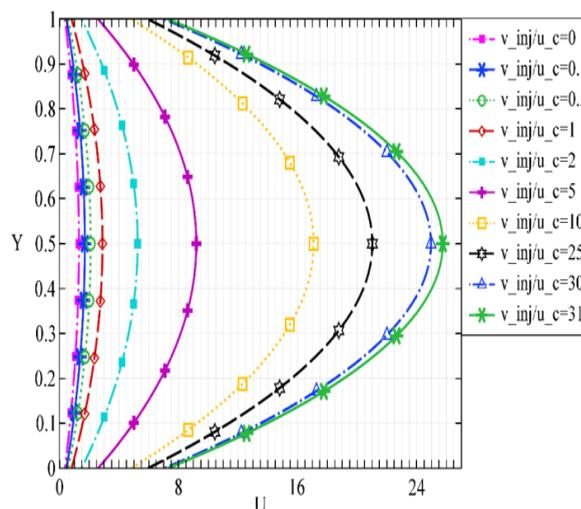
**Fig. 4** Dimensionless velocity profile at the vertical line  $X = 0.5L$  for input Reynolds number  $Re = 1$ ,  $\phi = 0.02$ ,  $B = 0.1$ , and different injection velocities.
