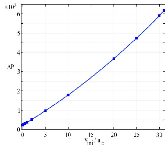
Fig. 10 Pressure drop for input Reynolds number  $Re = 1$ ,  $\phi = 0.02$ ,  $B = 0.1$ , and different injection velocities.
