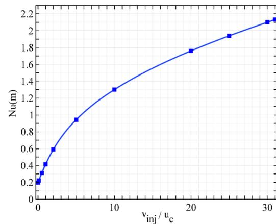
Fig. 9  $Nu_m$  calculated on the upper wall for input Reynolds number  $Re = 1$ ,  $\phi = 0.02$ ,  $B = 0.1$ , and different injection velocities.
