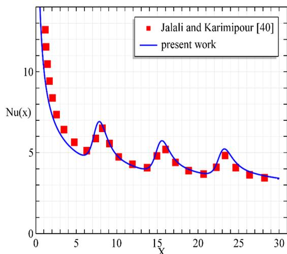
**Fig. 3**  $Nu_x$  for input and injection Reynolds numbers of 100,  $\phi = 0.02$ , and  $B = 0.1$ .
