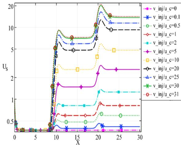
Fig. 7 Dimensionless slip velocity at the upper wall for input Reynolds number  $Re = 1$ ,  $\phi = 0.02$ ,  $B = 0.1$ , and different injection velocities.
