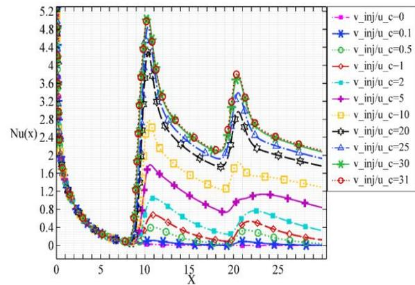
Fig. 8  $Nu_x$  calculated on the upper wall for input Reynolds number  $Re = 1$ ,  $\phi = 0.02$ ,  $B = 0.1$ , and different injection velocities.
