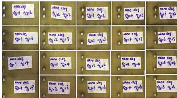
Fig. 2 Samples from laminate plate with different geometrical parameters.
