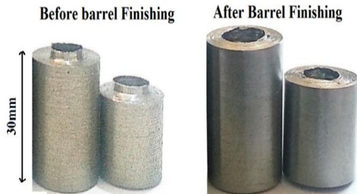
Fig. 4 Samples before and after barrel finishing. (Working time= 2 hrs., initial roughness= 8.96 \mu\text{m} , abrasive media: 75% steel balls and 25% aluminum oxide, final surface roughness= 3.75 \mu\text{m} ).
