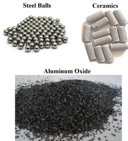
Fig. 3 Three types of used abrasive particles.
