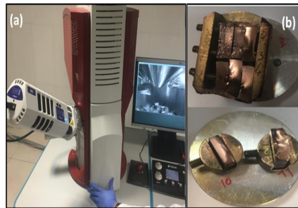
Fig. 1 (a): FESEM device, and (b): samples prepared for testing.
