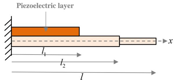
Fig. 1 A Nano-mechanical beam with a piezoelectric layer.
