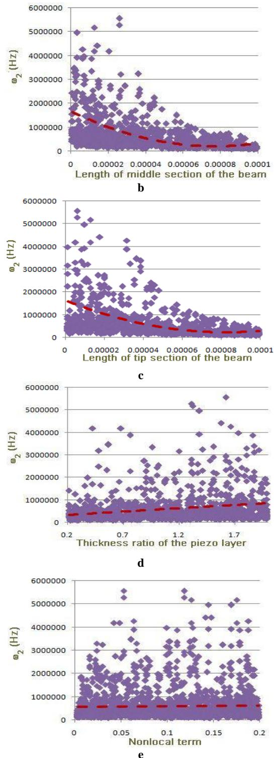
**Fig. 3** The second frequency versus length of the: (a): first section, (b): middle section, and, the second frequency versus length of the: (c): tip section, (d): piezo thickness ratio, and (e): nonlocal term
