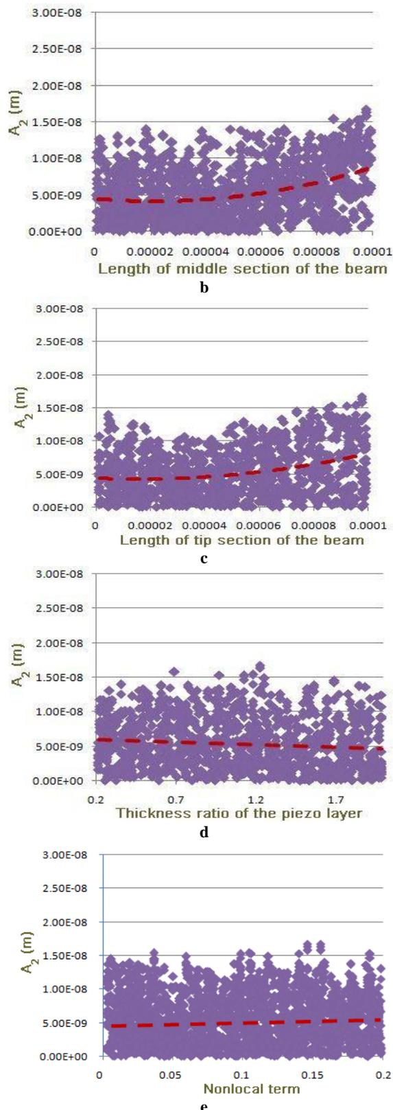
**Fig. 5** The second resonant amplitude versus length of the: (a): first section, (b): middle section, (c): tip section, and, the second resonant amplitude versus the: (d): piezo thickness ratio, (e): nonlocal term.
