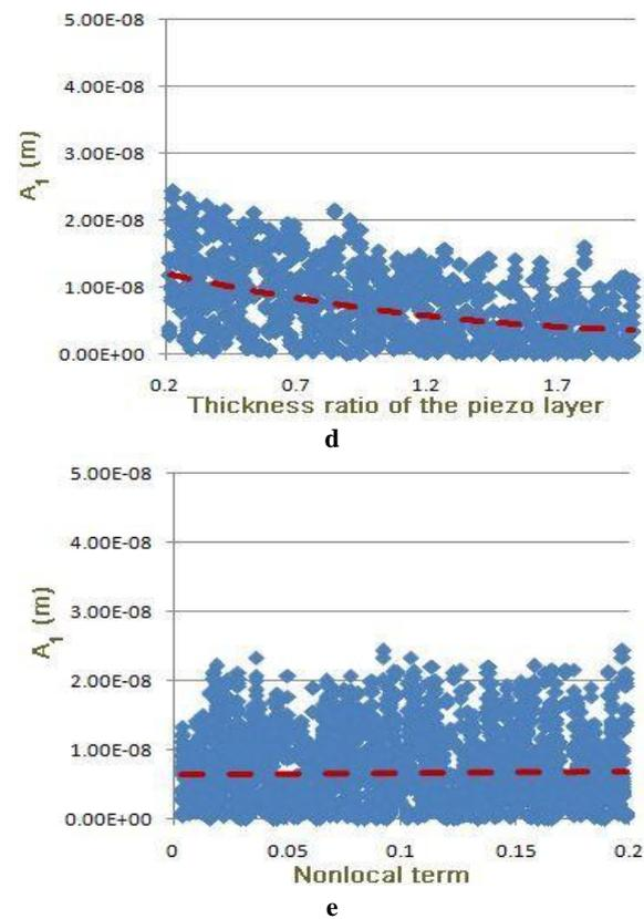
**Fig. 4** The first resonant amplitude versus length of the: (a): first section, (b): middle section, (c): tip section, and, the first resonant amplitude versus the: (d): piezo thickness ratio, (e): nonlocal term.
