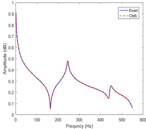
**Fig. 2** Comparing the point frequency response function of the degree of freedom 2 by two Exact and CMS methods.
