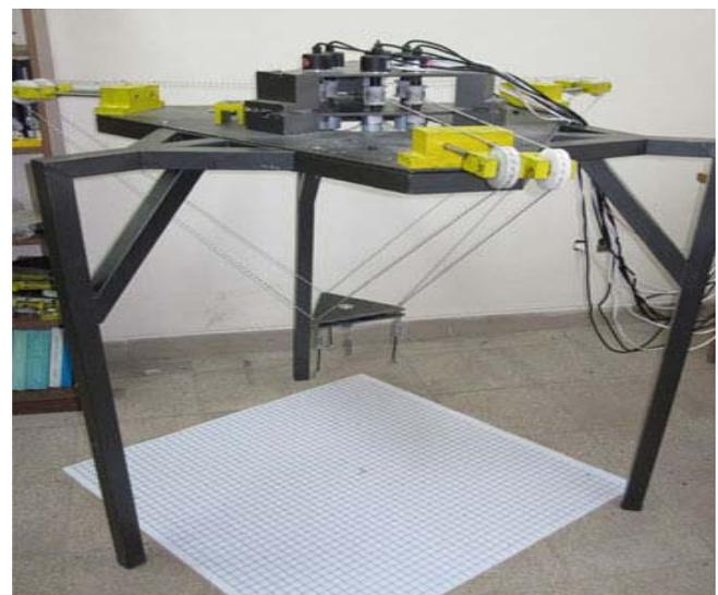
Fig. 5 Scheme of the designed IUST cable robot
