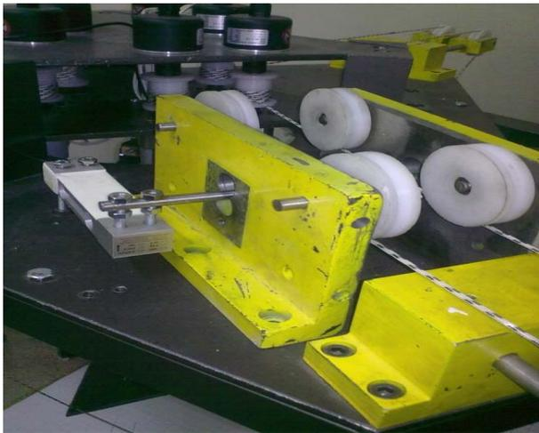
Fig. 2 Loadcell used as the tension sensing device
