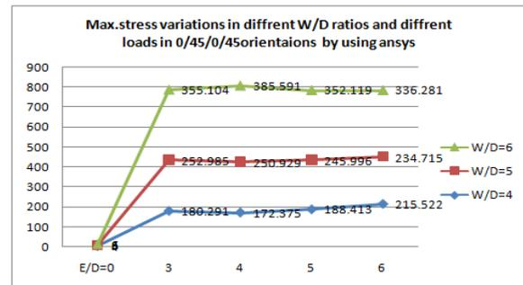
Fig. 13 The effect of width to diameter ratio on maximum stress (kg/ mm<sup>2</sup>) for [0/45/0/45] laminates
