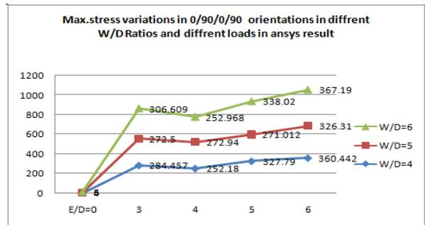
Fig. 5 The effect of edge distance to diameter ratio on the Max stress (kg/mm²) for [0/90/0/90] laminates
