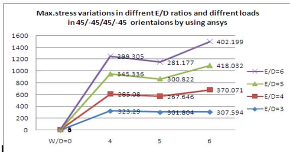
Fig. 8 The effect of edge distance to diameter ratio on maximum stress (kg/ mm<sup>2</sup>) for [45/-45/45/-45] laminates
