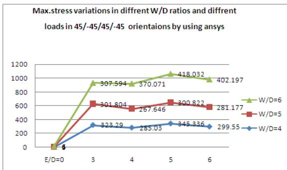
Fig. 9 The effect of width to diameter ratio on maximum stress (kg/ mm<sup>2</sup>) for [45/-45/45/-45] laminates
