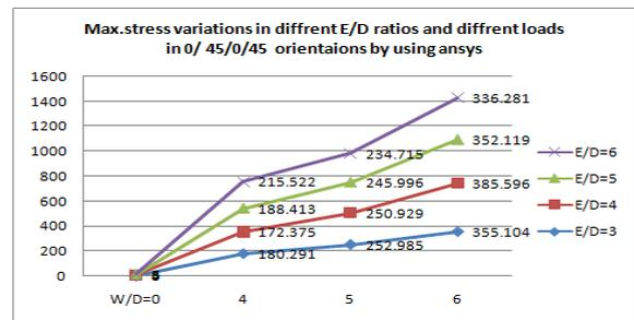
Fig. 12 The effect of edge distance to diameter ratio on maximum stress (kg/ mm<sup>2</sup>) for [45/-45/45/-45] laminates
