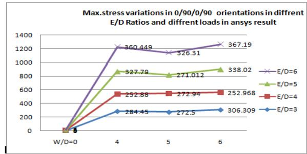
Fig. 4 The effect of width to diameter ratio on the Max stress (kg/mm²) at failure for [0/90/0/90] laminates
