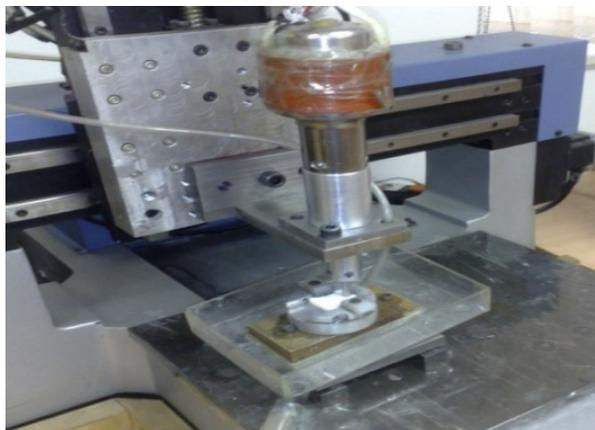
Fig. 2 Experimental set-up for ultrasonic machining
