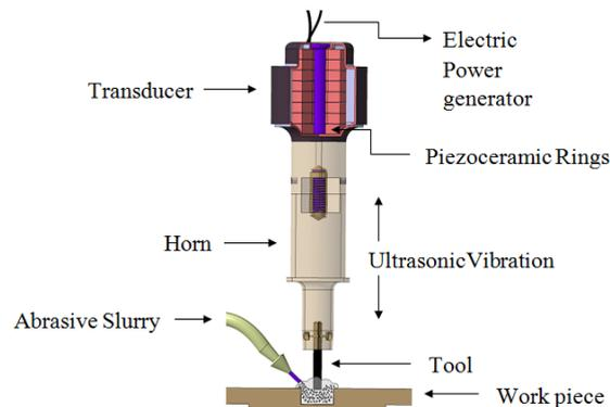
Fig. 1 Schematic view of a USM setup
