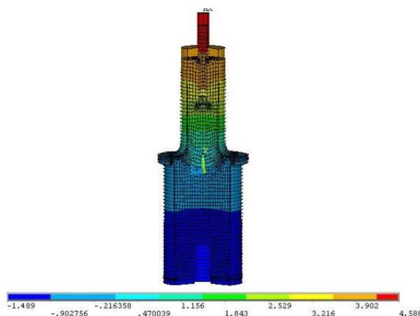
Fig. 3 Longitudinal amplification diagram of ultrasonic head
