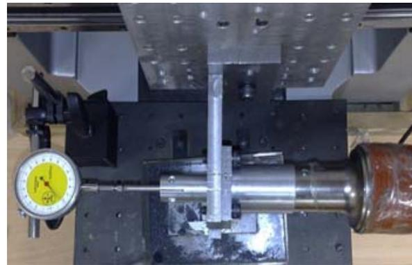
Fig. 4 Measuring method of vibration amplitude
