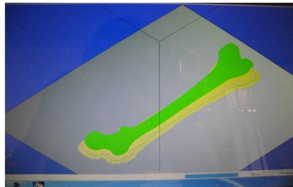
Fig. 13 Layered model in the RP system's software [27]
