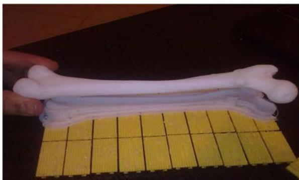
Fig. 16 Part's separation from its support [27]
