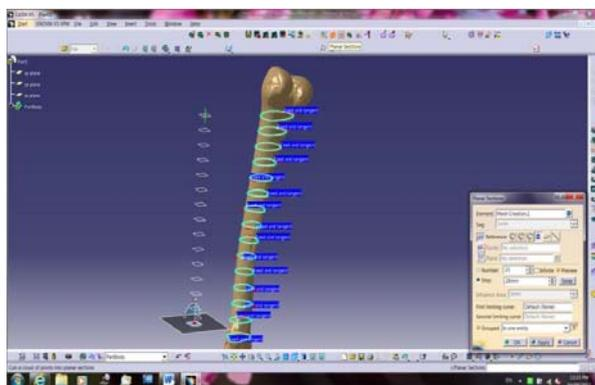
Fig. 11 Contour generation of meta and diaphysis [27]
