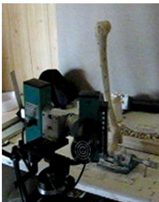
Fig. 6 Optical measurement of femur bone [27]
