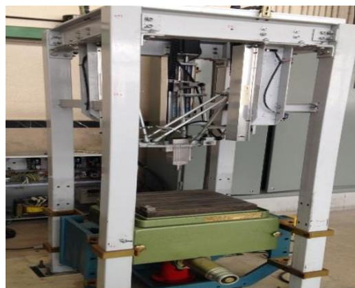
**Fig. 1** 2-PR(Pa)U-2-PR(Pa)R parallel mechanism with 4 degrees of freedom
