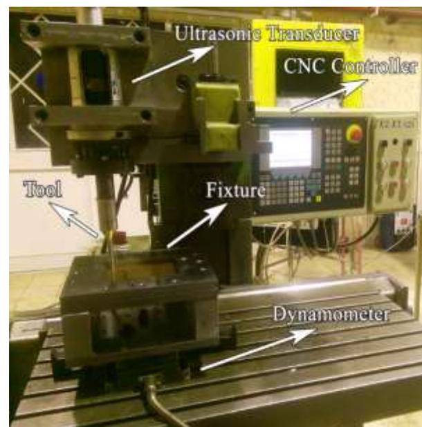
**Fig. 1** The experimental setup for the incremental forming process.
