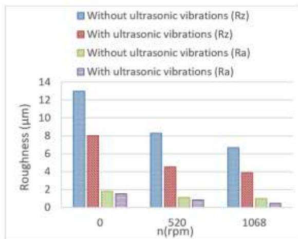
Fig. 6 Effect of rotational speed and ultrasonic vibrations on the surface roughness.
