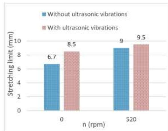
Fig. 9 Results of stretching limit in straight groove test.
