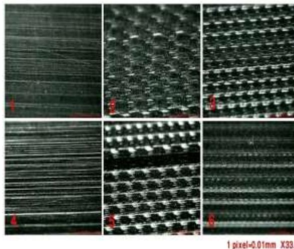
**Fig. 5** Effect of rotational speed and ultrasonic vibrations on the surface topography (picture number is coordinate with test number in Table 1).
