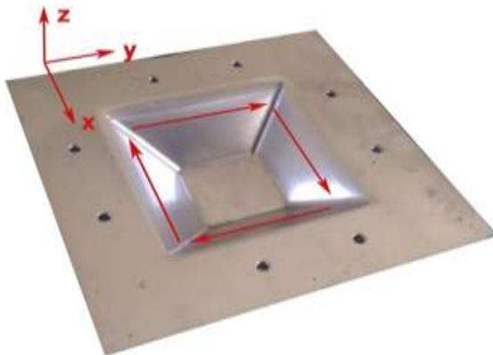
Fig. 2 Sample geometry and tool path.
