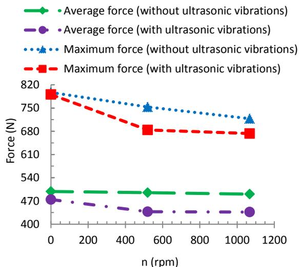
**Fig. 4** Comparison of forming force according to the rotational speed and ultrasonic vibrations.
