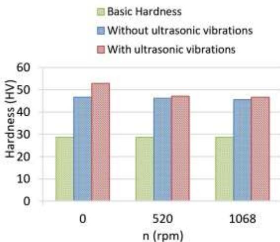
Fig. 7 Effects of ultrasonic vibrations and rotational speed on the surface hardness.
