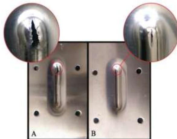
Fig. 8 Samples of the stretching limit test: (A): 520 (rpm) rotational speed with ultrasonic vibrations and (B): without rotation and ultrasonic vibrations.
