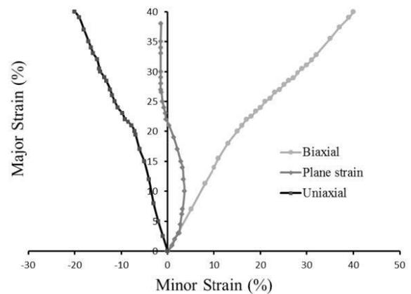
**Fig. 11** The strain path of three distinct configurations in the EHF process with incremental increasing of the discharge voltage.
