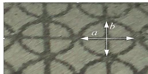
Fig. 2 Specimen after tensile stress test: (a): larger diameter and (b): smaller diameter, of the deformed grid.
