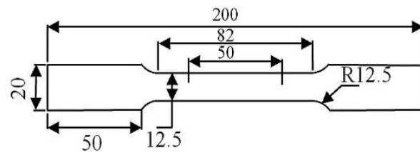
Fig. 1 Dimensions of uniaxial tensile test specimens (mm) [14].
