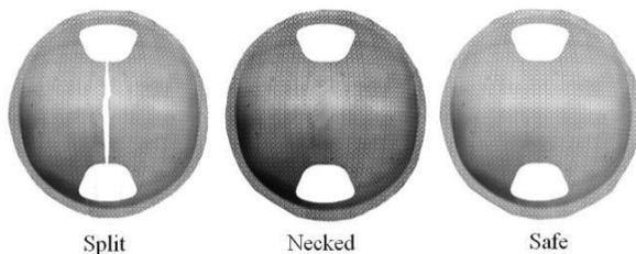
**Fig. 10** Safe, necked and split (failure) modes of the EHF-formed parts.
