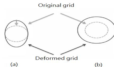
Fig. 3 Two different strain distribution of deformed specimens: (a): plane strain ( $\epsilon_1 > 0, \epsilon_2 = 0$ ) and (b): biaxial ( $\epsilon_1 = \epsilon_2 > 0$ ) states.
