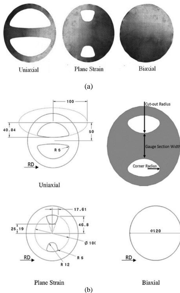
**Fig. 6** (a): Different configurations and dimensions of initial blank to generate distinct major strains ratio (mm) [8] and (b): blanks’ configuration of Brass 260 and Al5182-O sheets in hydrodynamic and EHF processes.
